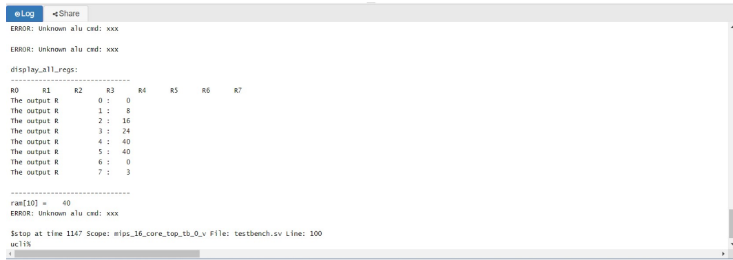
Figure 4.4: Simulation of processor using testbench
