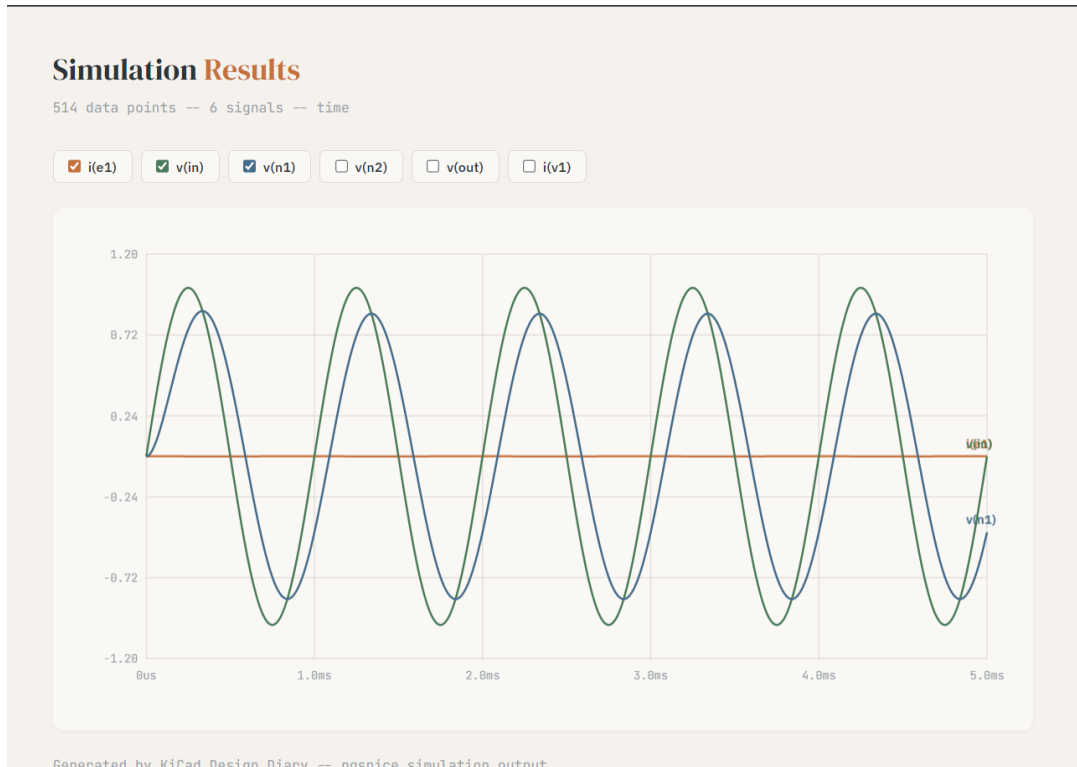
Figure 6.2: Interactive waveform view after a successful NGSpice run (Sallen–Key validation).
