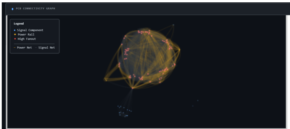
Figure 5.17: Stickhub Connectivity Graph: U1 shown as red star due to high fanout from 7 USB port connections
