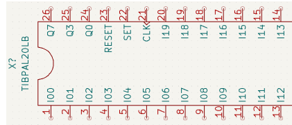
Figure 6.1: Subcircuit of TIBPAL20L8
