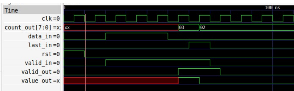
Figure 4.32: Digital Gate-Level Timing Waveforms Visualized inside GTKWave
