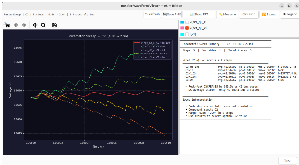
Figure 5.5: Parametric sweep of the Two-Stage Stagger-Tuned Amplifier varying the tuning capacitor C2 across five values (0.8 nF, 1.0 nF, 1.2 nF, 1.5 nF, 2.0 nF). Each step shifts the Stage 1 resonant frequency, showing how capacitor value controls the stagger-tuning effect. Five overlaid traces appear in distinct colours. The stats panel shows per-step average and peak-to-peak values.
