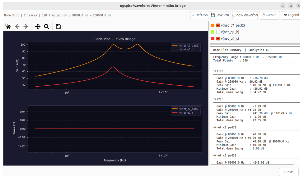
Figure 5.8: Bode plot of the Two-Stage Stagger-Tuned Amplifier from the AC analysis. The upper subplot shows gain in dB vs. frequency (semilog). The two gain peaks from the two stagger-tuned stages are visible at approximately 139 kHz and 167 kHz. The lower subplot shows phase in degrees. The stats panel shows peak gain, frequency of peak, and total gain swing.
