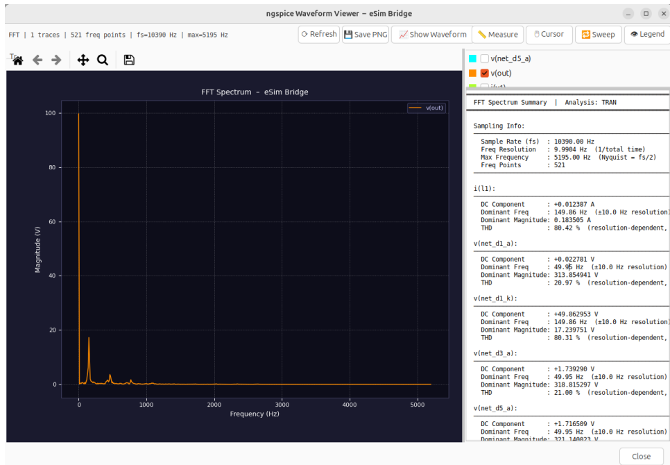
Figure 5.4: FFT spectrum of the rectifier output v(out) . The dominant spectral component at approximately 150 Hz corresponds to the 6-pulse ripple frequency ( 3 \times 50 Hz). The DC component and higher harmonics are also visible. The stats panel shows dominant frequency, peak magnitude, and THD.
