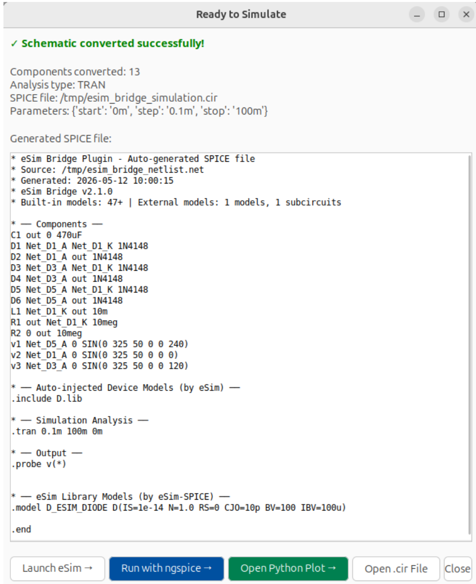
Figure 4.6: The SimulationReadyDialog showing the auto-generated SPICE file for the Three-Phase Bridge Rectifier. The preview panel displays the component lines (D1-D6, C1, L1, R1, R2, V1-V3), auto-injected diode model ( .model D_ESIM_DIODE ), and the .control block with the transient analysis command. The four action buttons are visible at the bottom right.
