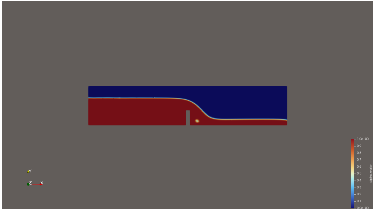
Figure 4: Phase fraction \alpha in the weir-only case at steady state
