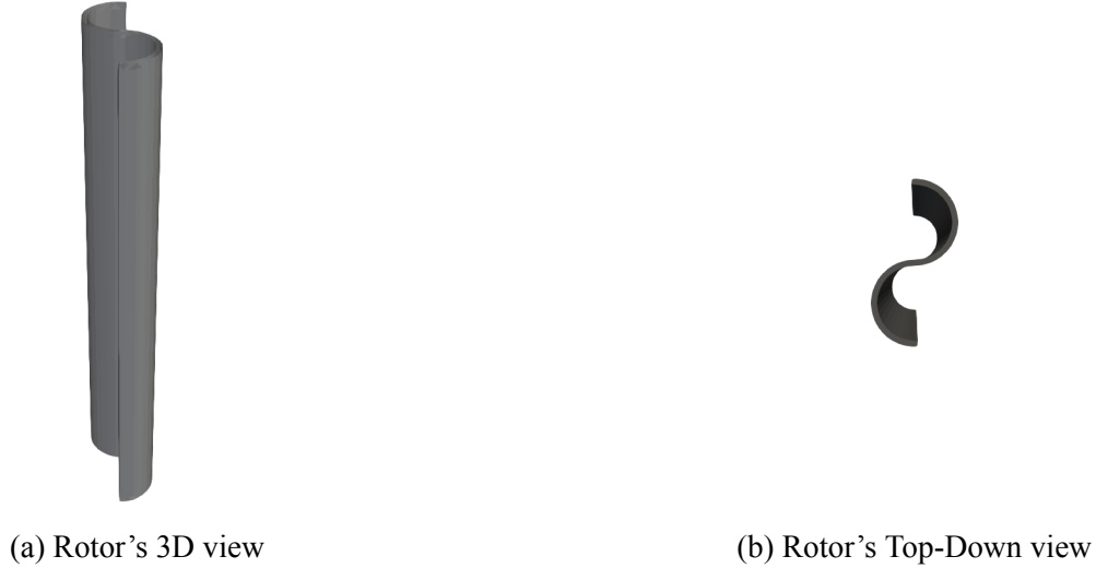
Figure 2: Savonius rotor CAD geometry with characteristic dimensions H = 300\text{mm} , D = 82\text{mm}
