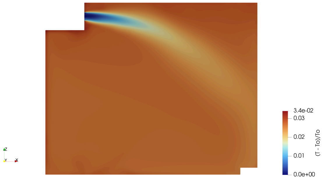
Fig. 3. Contour of the CFD simulation results for the reference case. (a) contour location; (b) dimensionless velocity magnitude; and (c) dimensionless air temperature.
