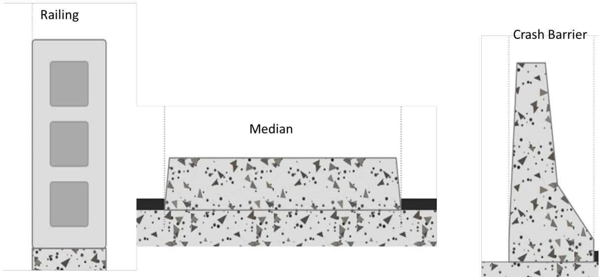
Figure 4.5: 2D CAD visualization of crash barriers, medians, and railing systems
