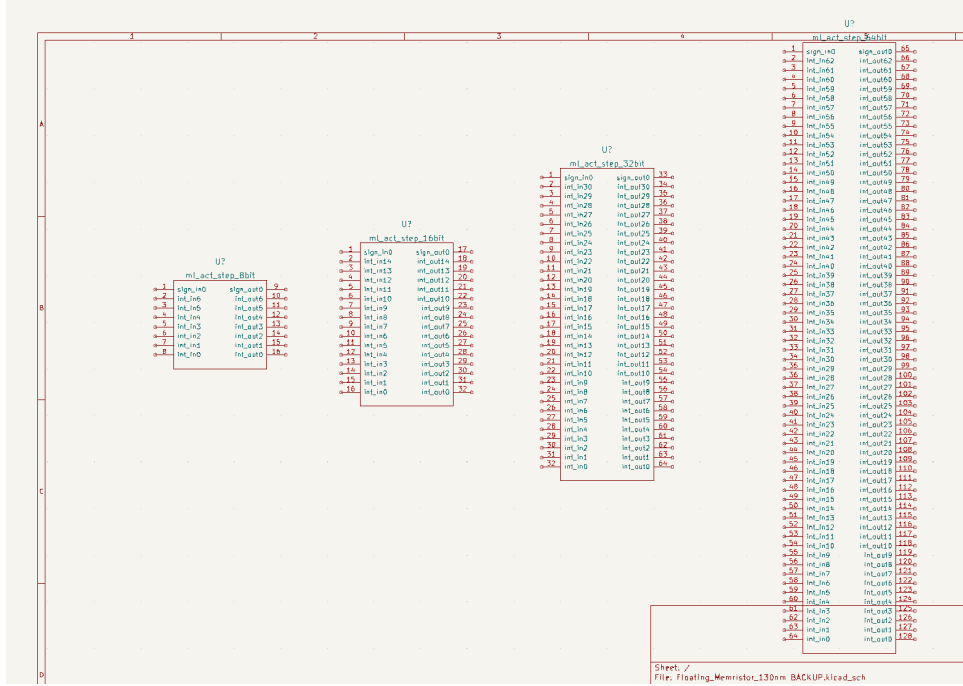
Figure 25: The generated KiCad schematic symbols for the Binary Step IP suite. Notice the absence of fractional pins, optimizing the block strictly for pure integer processing.
