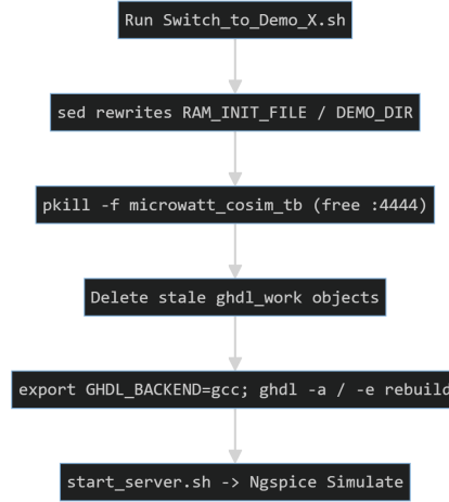
Figure 78: Demonstration-switching sequence: rewrite the firmware path, kill any stale server holding the socket, purge old GHDL work objects, and re-elaborate under the GCC backend before re-launching the simulation.
