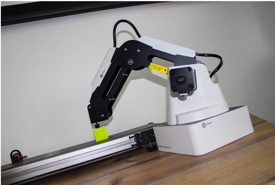
Figure 1: Simulation of a desktop-class Dobot platform integrated into an automated production setup.
