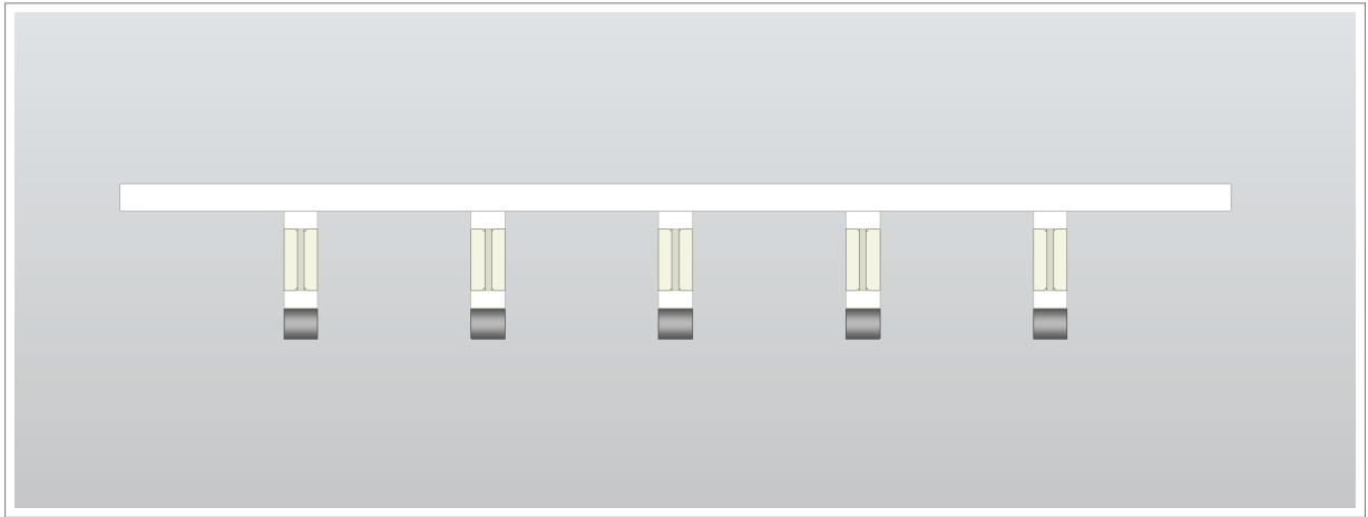
Figure 3.11: Deck slab positioned on plate girders showing complete deck–girder assembly - Front View
