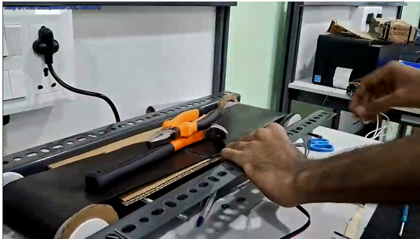
Figure 3.2: The Phase 2 prototype featuring the slotted angle iron chassis, the upgraded Rexine synthetic belt, and the integrated cardboard slider bed utilized to provide rigid vertical payload support.
