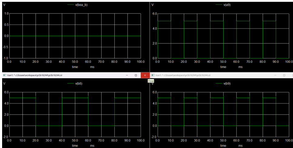
Figure 4.32: Input and output Waveform of PI3B3861
