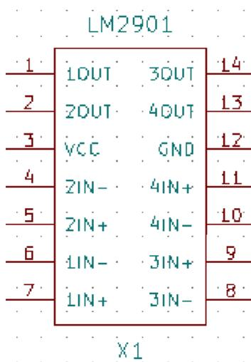
Figure 4.4.1.1: Pin Configuration of LM2901
