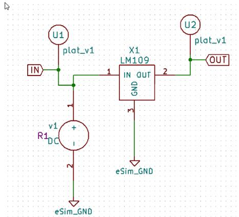
Figure 4.2.3.1: Test Circuit of the LM109
