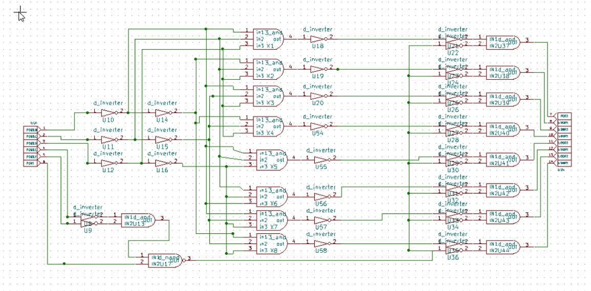
Figure 5.2.2.1: Subcircuit layout of the MC74HC238
