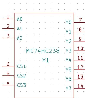
Figure 5.2.1.1: Pin Configuration of MC74HC238
