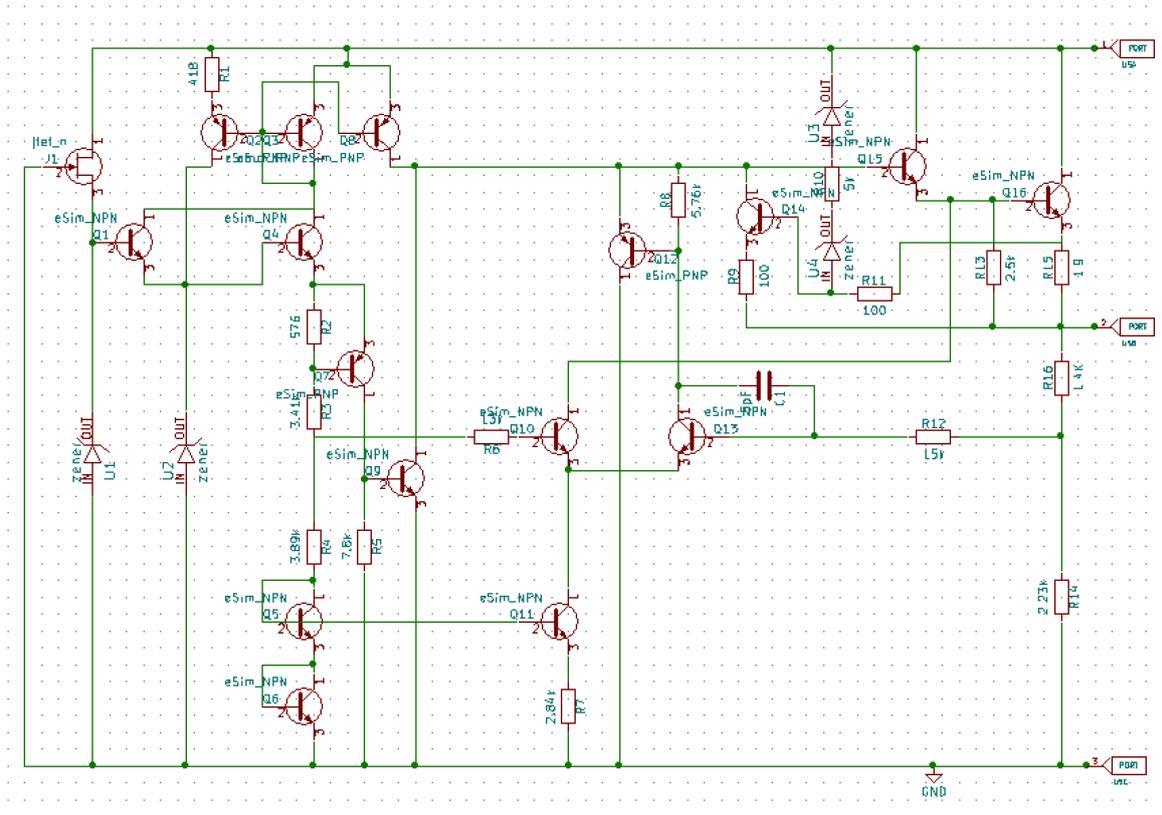
Figure 4.1.2.1: Subcircuit layout of the LM342 voltage regulator.
