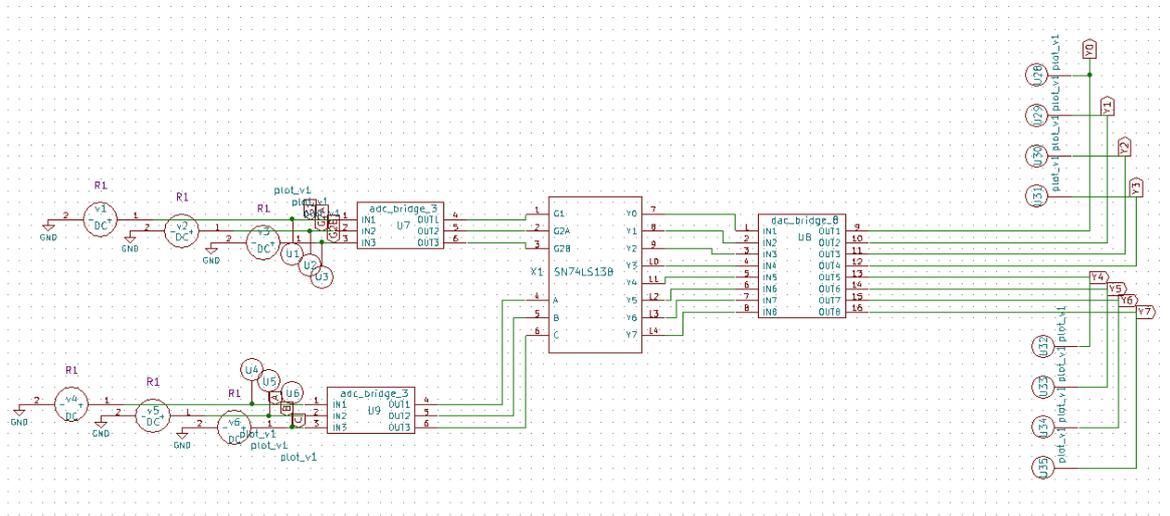
Figure 5.7.3.1: Test circuit layout of the SN74LS138
