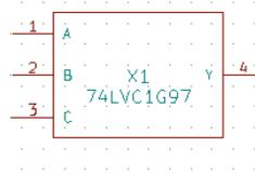
Figure 5.4.1.1: Pin Configuration of 74LVC1G97
