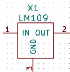
Figure 4.2.1.1: Pin Configuration of LM109
