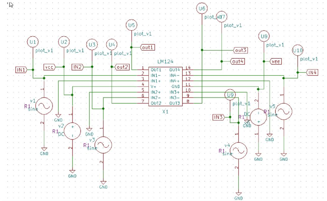
Figure 4.3.3.1: Test Circuit of LM124
