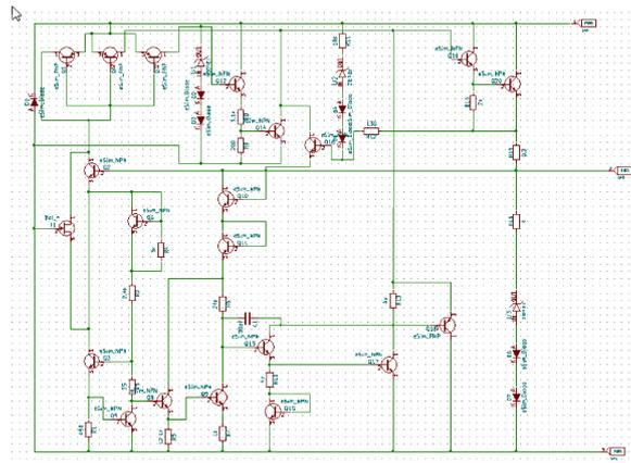
Figure 4.2.2.1: Subcircuit layout of the LM109
