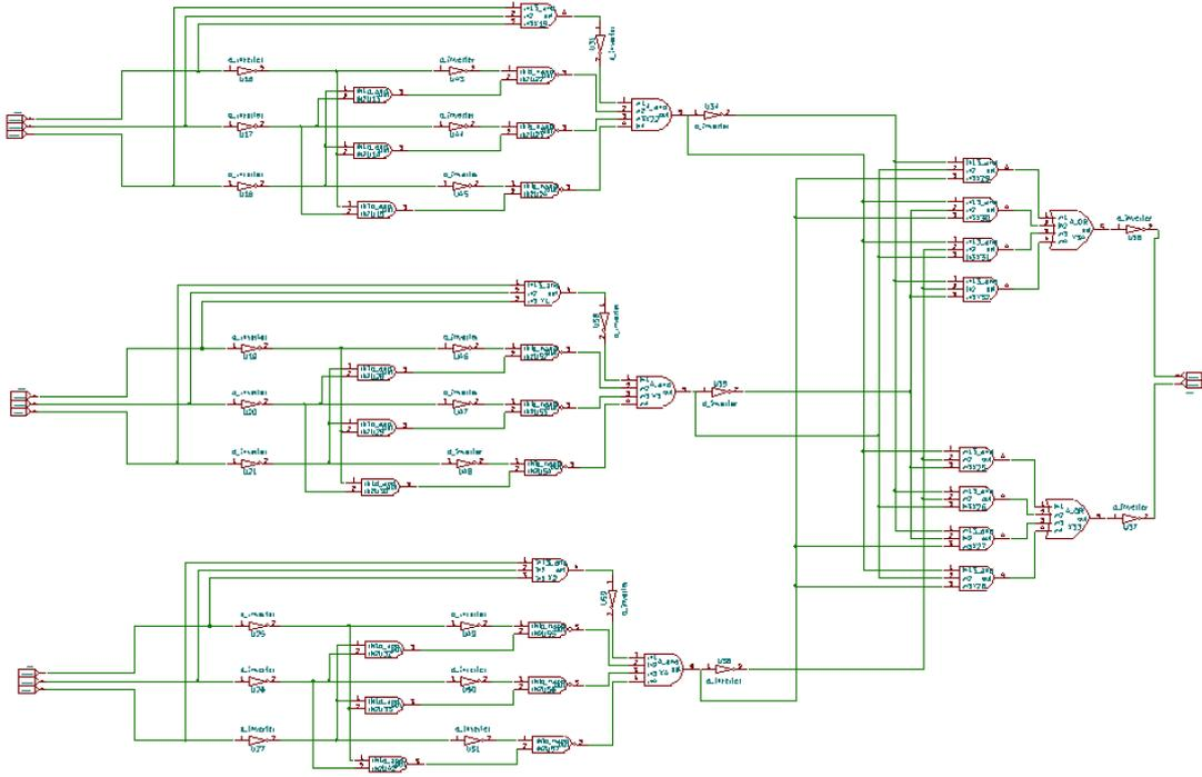
Figure 5.1.2.1: Subcircuit layout of the SN74ALS280
