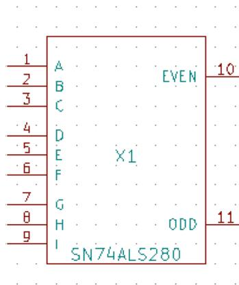
Figure 5.1.1.1: Pin Configuration of SN74ALS280
