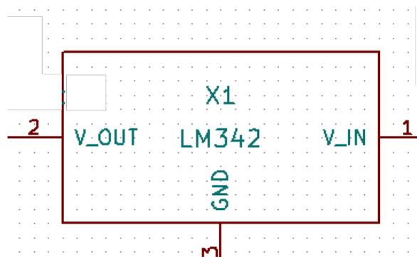
Figure 4.1.1.1: Pin configuration of the LM342 voltage regulator.
