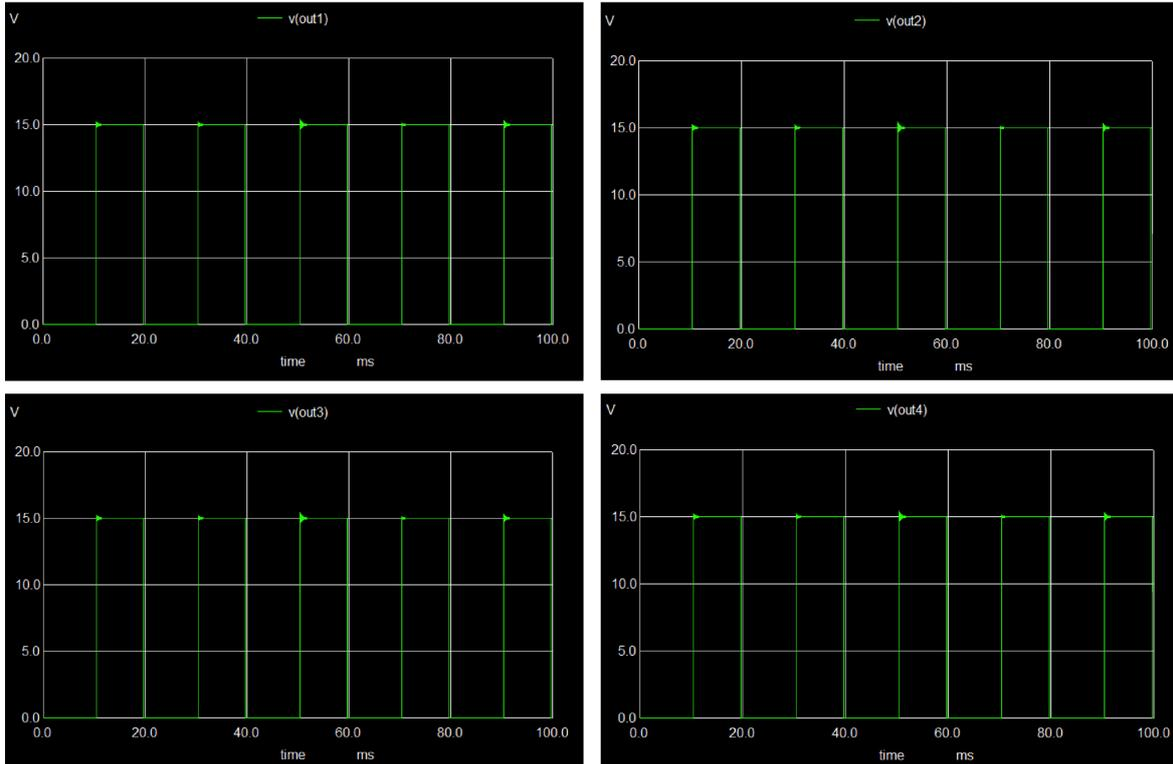
Figure 4.4.5.1: Output Wave form of LM2901
