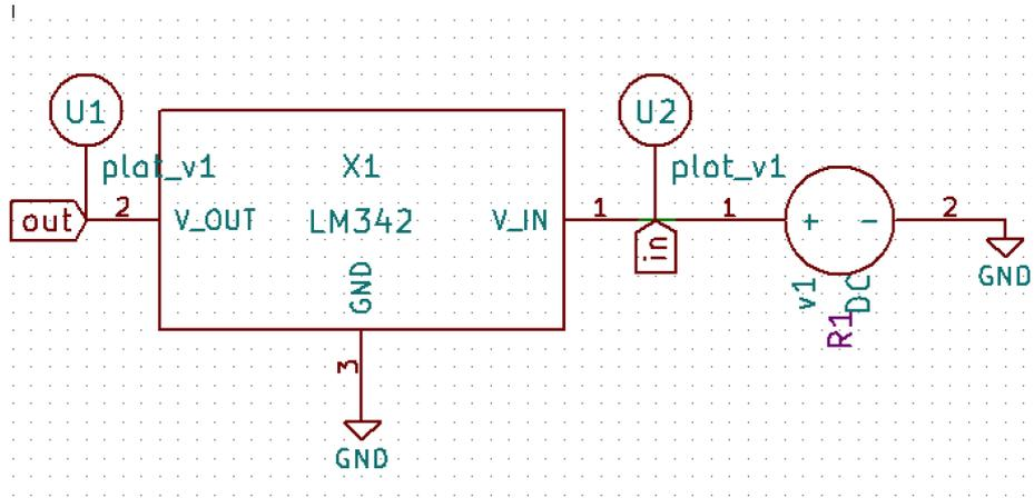
Figure 4.1.3.1: Test circuit setup for the LM342 voltage regulator.
