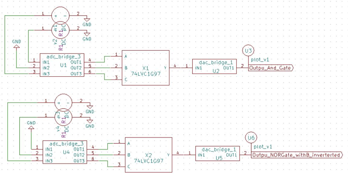
Figure 5.4.3.1: Test Circuit layout of the 74LVC1G97
