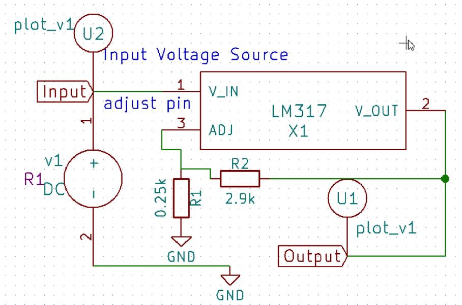
Figure 4.5.3.1: Test circuit setup for the LM317 voltage regulator.
