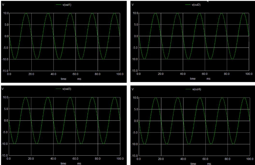
Figure 4.3.5.1: Output Wave form of LM124
