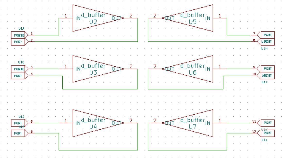
Figure 5.5.2.1: Subcircuit layout of the CD4050
