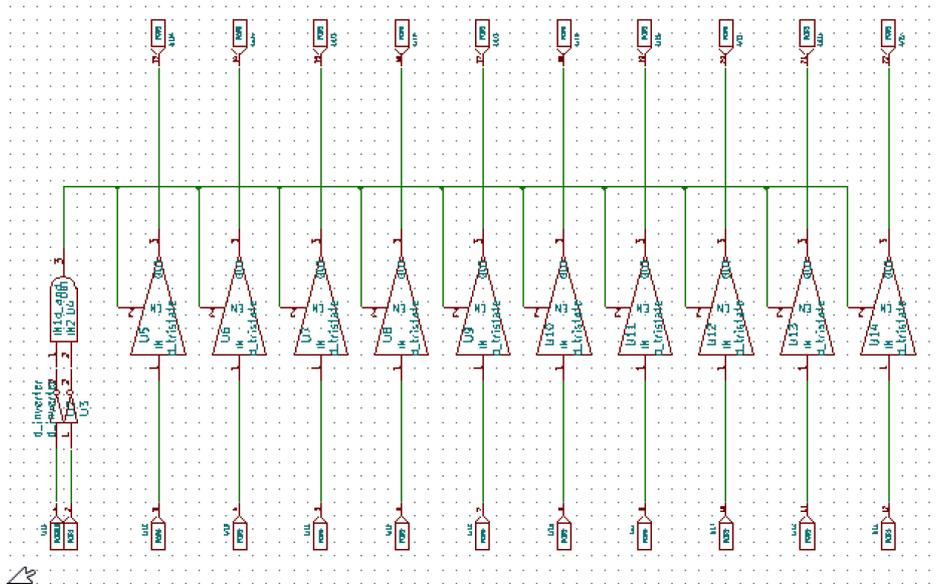
Figure 5.6.2.1: SUB circuit layout of the CY74FCT827ATQCT
