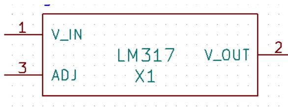
Figure 4.5.1.1: Pin configuration of the LM317 voltage regulator.
