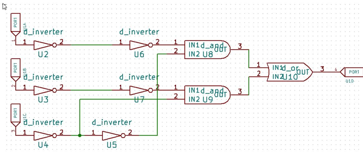
Figure 5.4.2.1: Subcircuit layout of the 74LVC1G97
