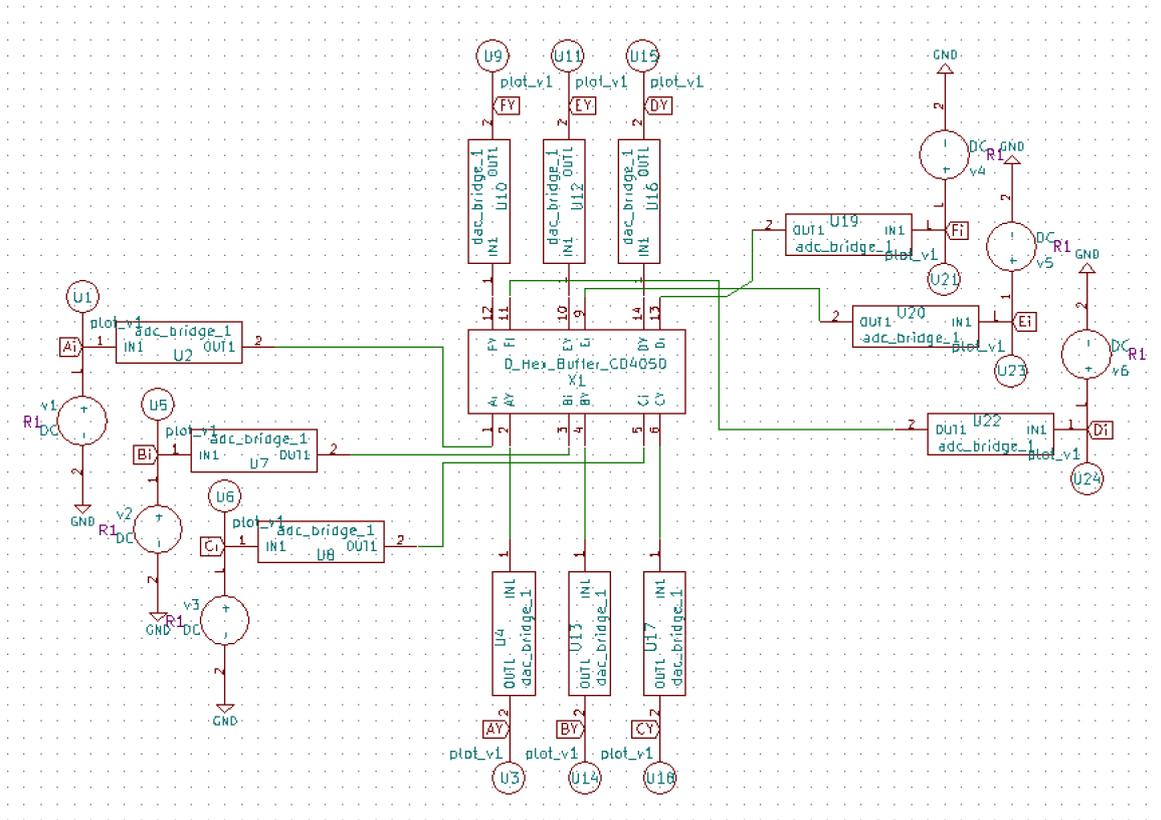
Figure 5.5.3.1: Test circuit layout of the CD4050
