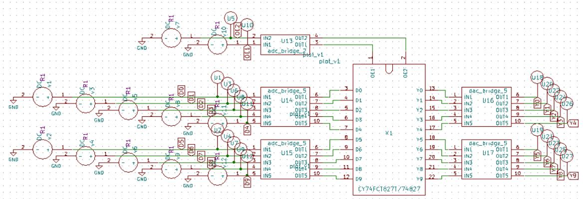
Figure 5.6.3.1: Test circuit layout of the CY74FCT827ATQCT
