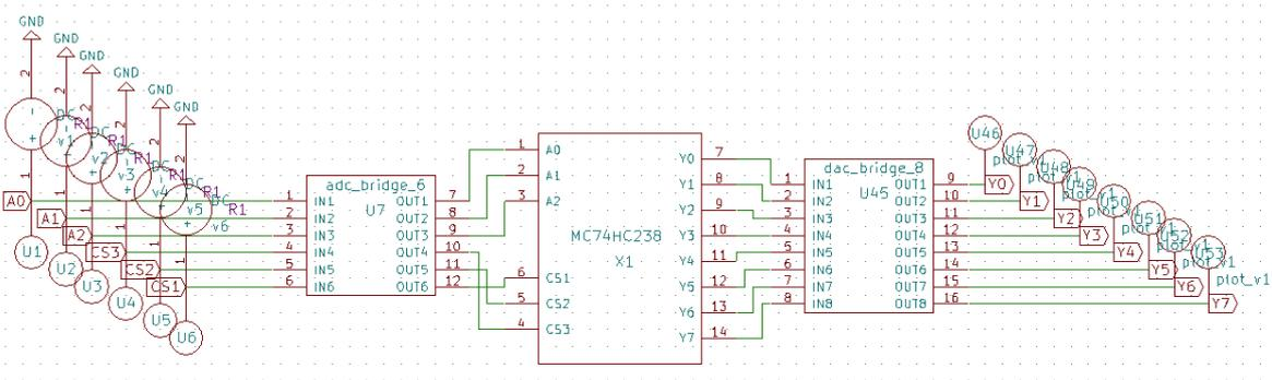
Figure 5.2.3.1: Test Circuit layout of the MC74HC238
