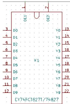
Figure 5.6.1.1: Pin Configuration of the CY74FCT827ATQCT
