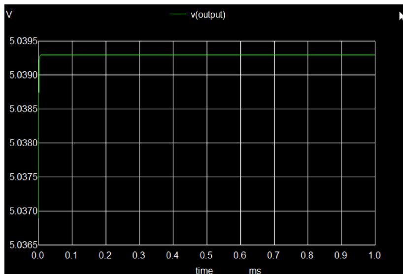
Figure 4.5.5.1: Output waveform of the LM317 voltage regulator.
