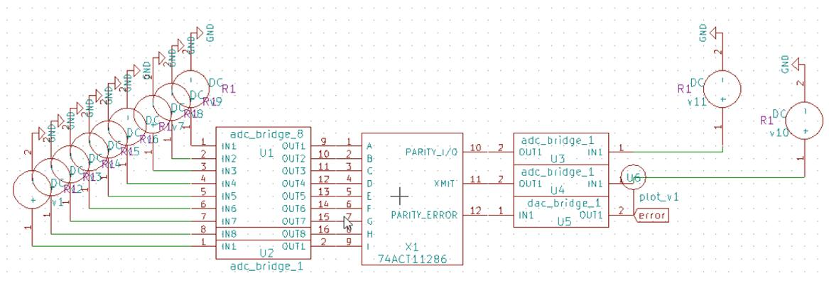
Figure 5.3.3.1: Test Circuit layout of 74ACT11286
