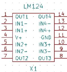
Figure 4.3.1.1: Pin Configuration of LM124
