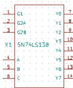
Figure 5.7.1.1: Pin Configuration of SN74LS138
