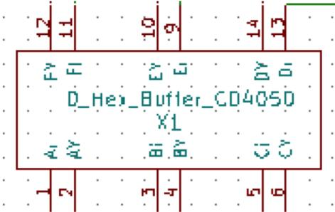
Figure 5.5.1.1: Pin Configuration of the CD4050
