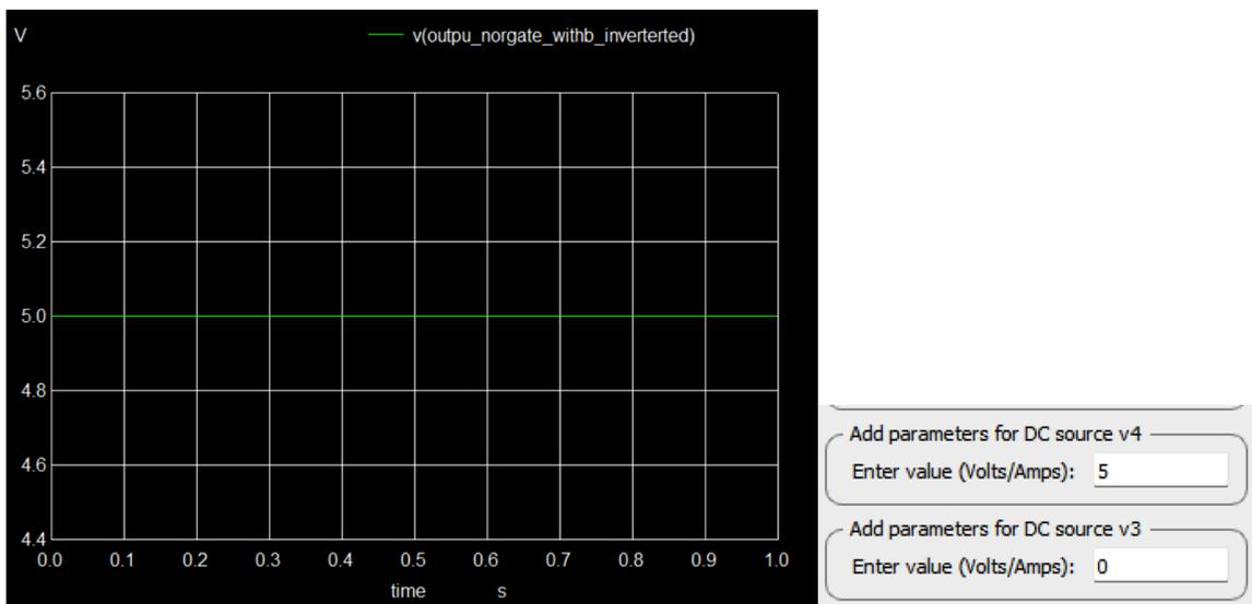
Figure 5.4.5.2: Output Waveform for 74LVC1G97
