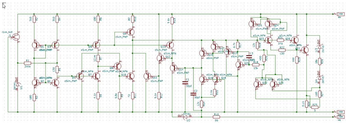
Figure 4.5.2.1: Subcircuit layout of the LM317 voltage regulator.
