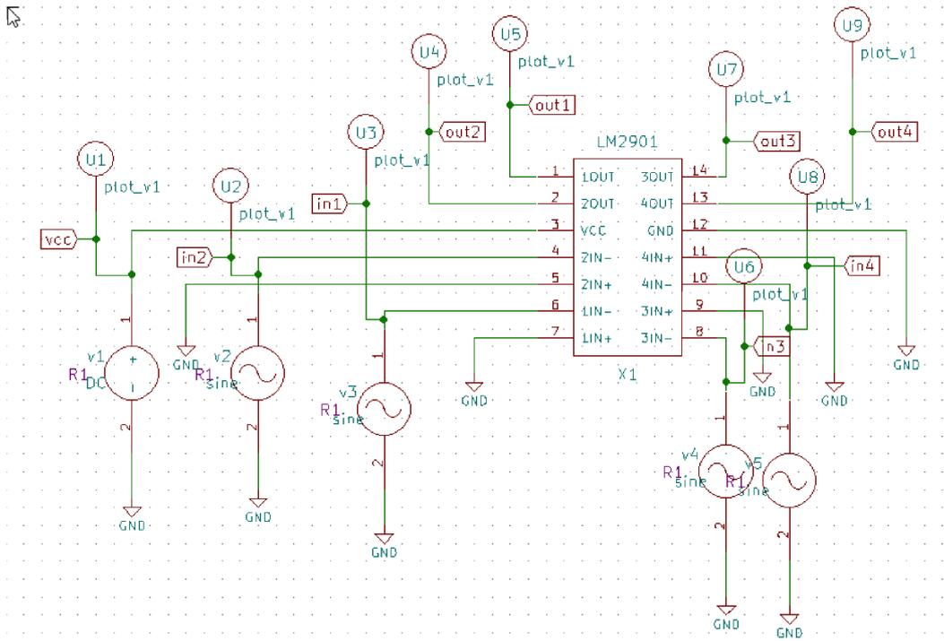
Figure 4.4.3.1: Test Circuit Layout of the LM2901
