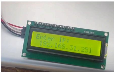
Fig 2.1: IP address in LCD
