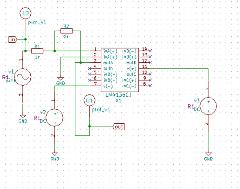
Figure 3.69: LM4136 Test Circuit(Inverting Amplifier)
