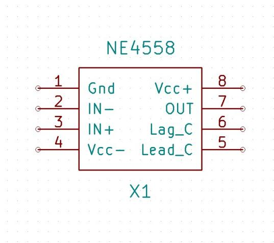
Figure 3.189: NE4558 Pin Diagram
