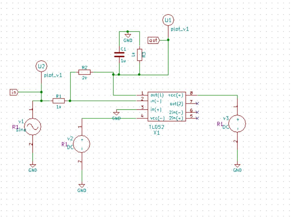
Figure 3.84: TL052 Test Circuit(Inverting Amplifier)
