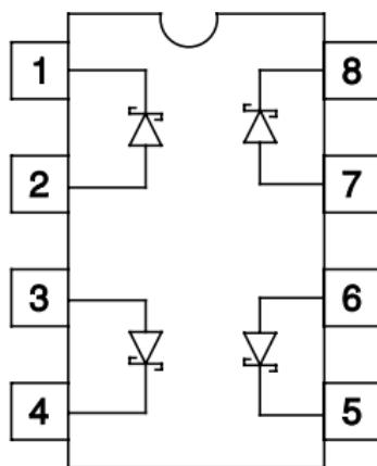
Figure 3.112: UC3611 Pin Diagram
