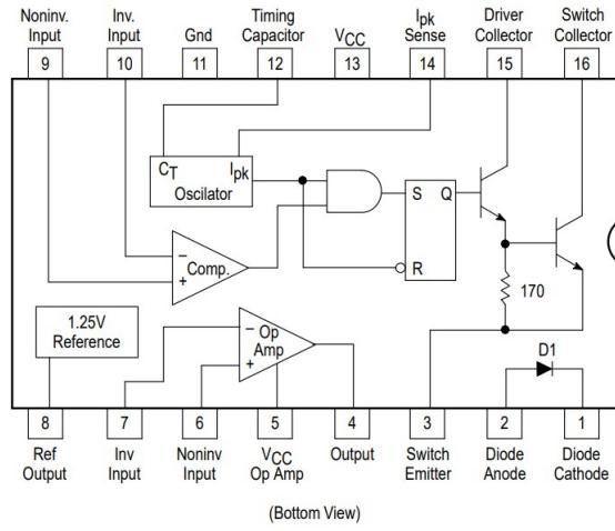
Figure 3.197: uA78S40 Pin Diagram
