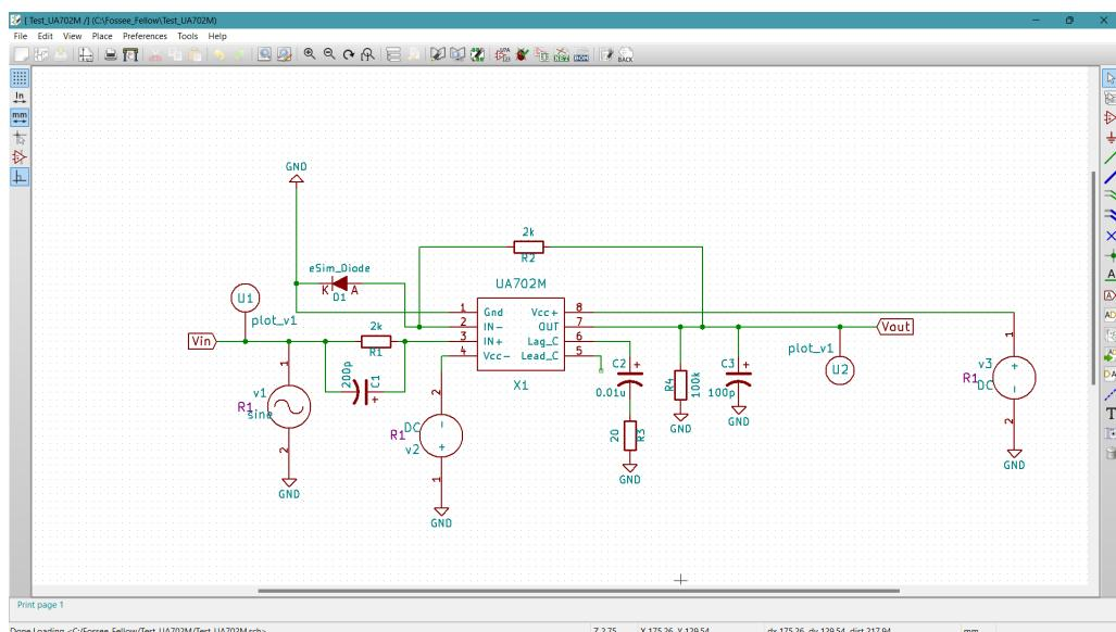
Figure 3.155: UA702 Test Circuit(Unity Gain Amplifier)
