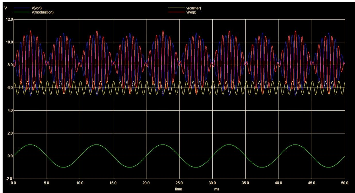
Figure 3.144: Output Suppressed Carrier Modulator
