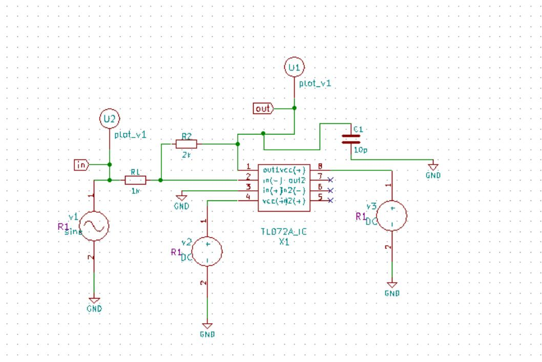
Figure 3.94: TL072 Test Circuit
