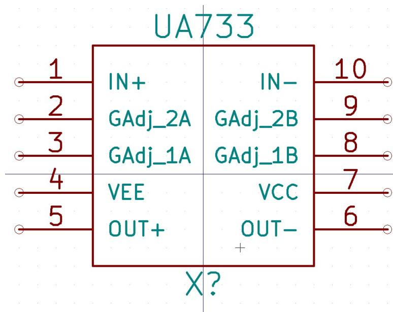
Figure 3.165: UA733 Pin Diagram
