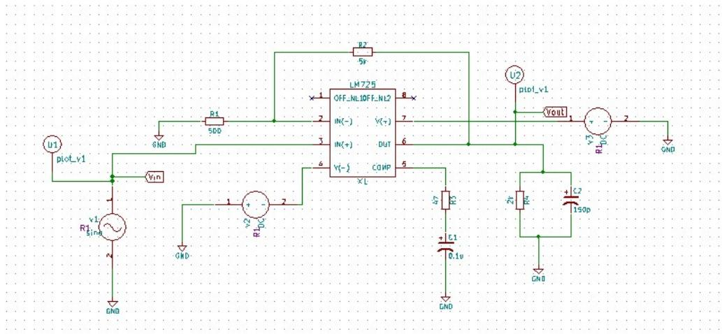
Figure 3.28: LM725 Test Circuit(Non-Inverting Amplifier)
