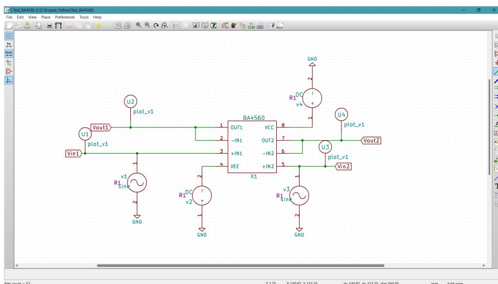
Figure 3.163: BA4560 Test Circuit(Non-Inverting Amplifier)
