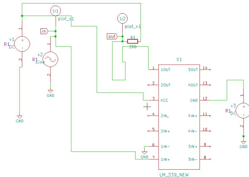
Figure 3.134: LM339 Test Circuit
