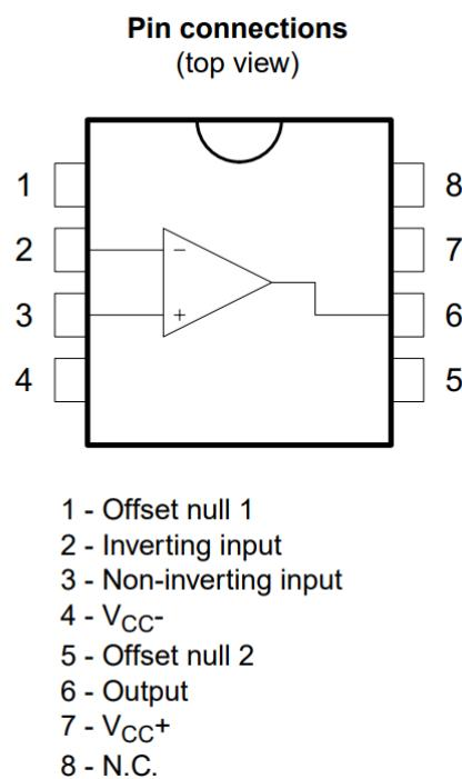
Figure 3.97: LF351 Pin Diagram
