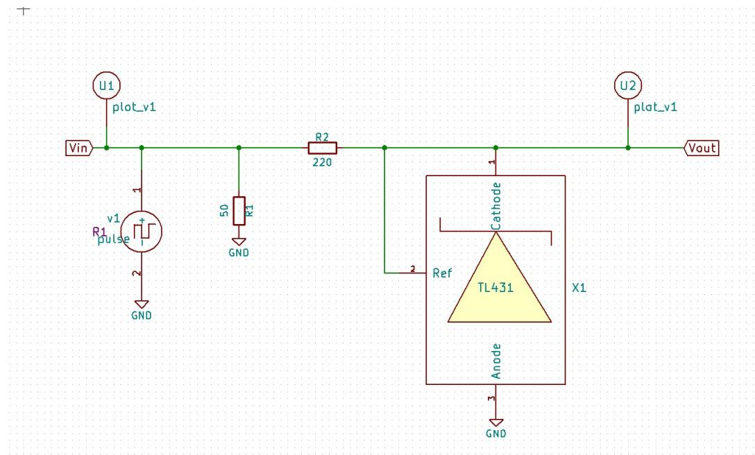
Figure 3.159: TL431 Test Circuit(Pulse Response)
