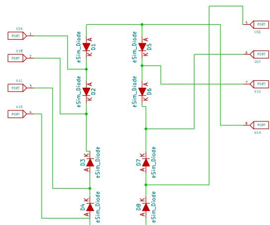
Figure 3.123: UC3610 Schematic
