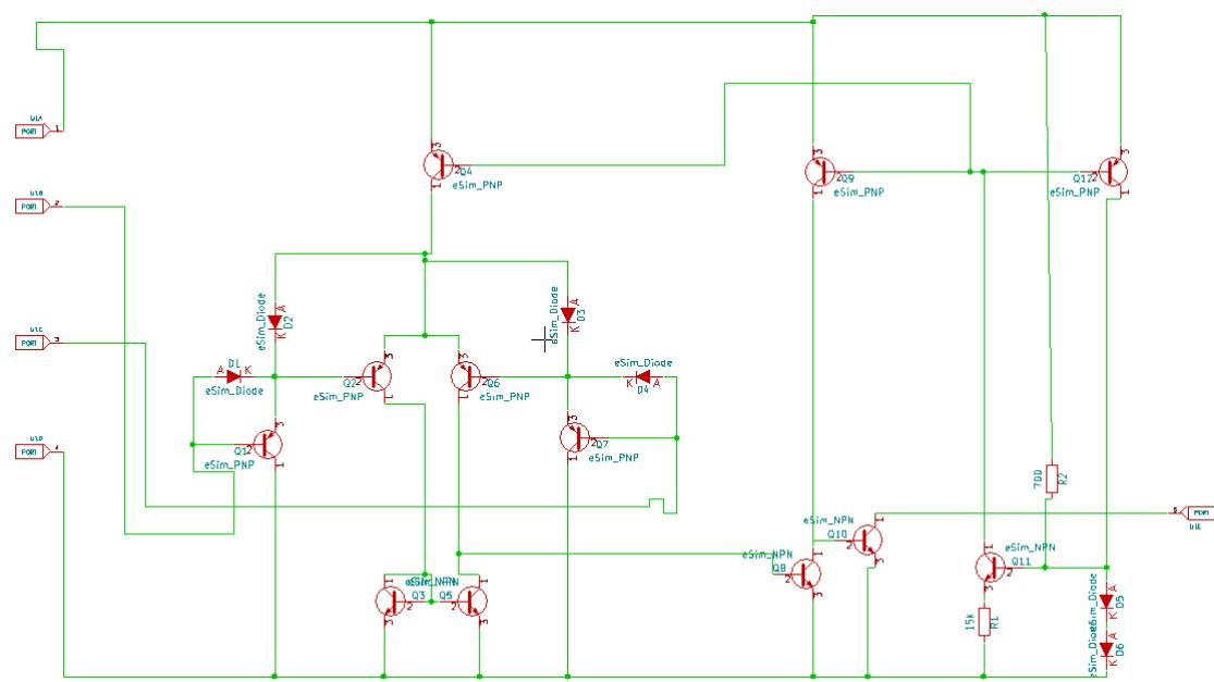
Figure 3.133: LM339 Schematic of a single pair
