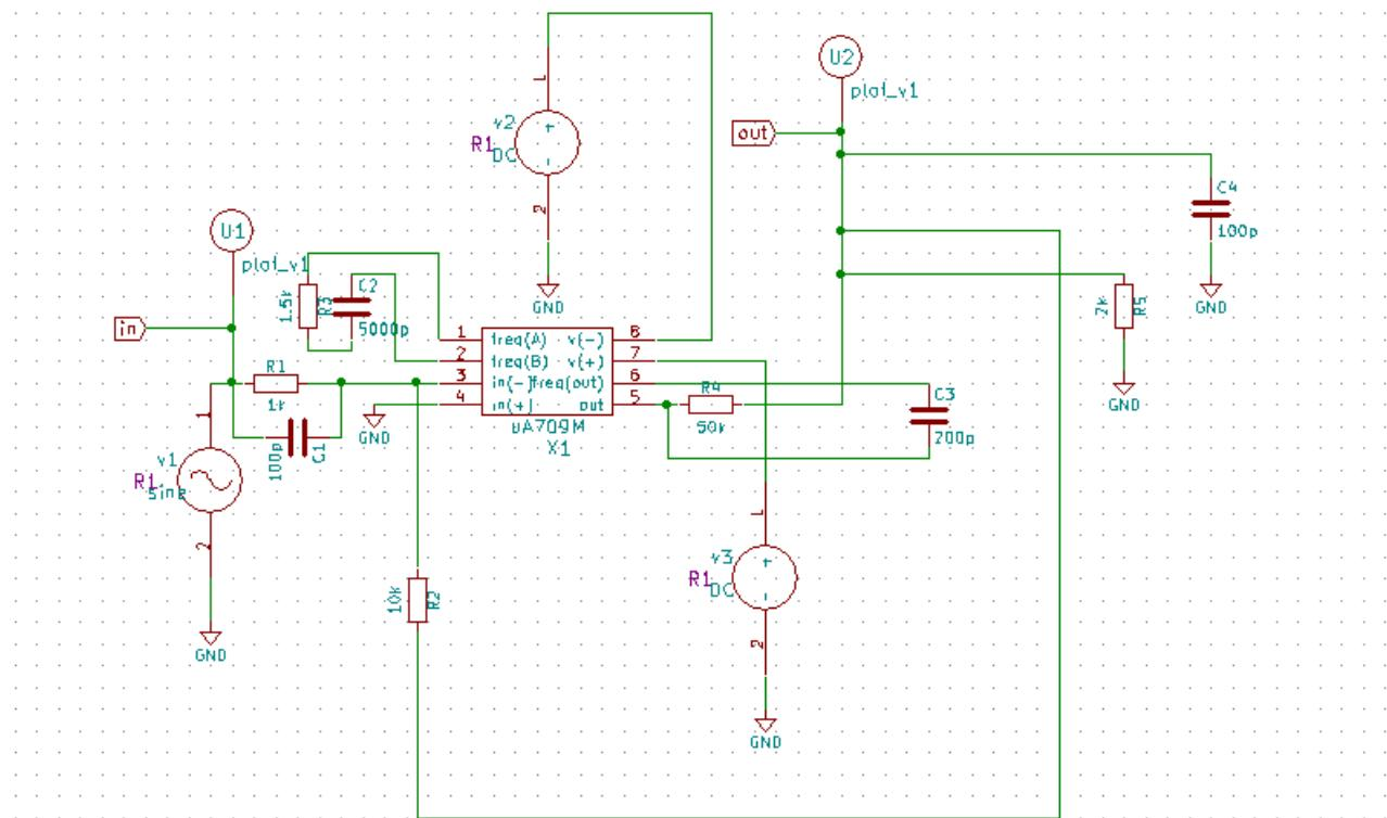
Figure 3.55: UA709 Test Circuit (Inverting Amplifier)
