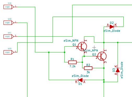
Figure 3.103: ULN2001 Schematic of a single pair
