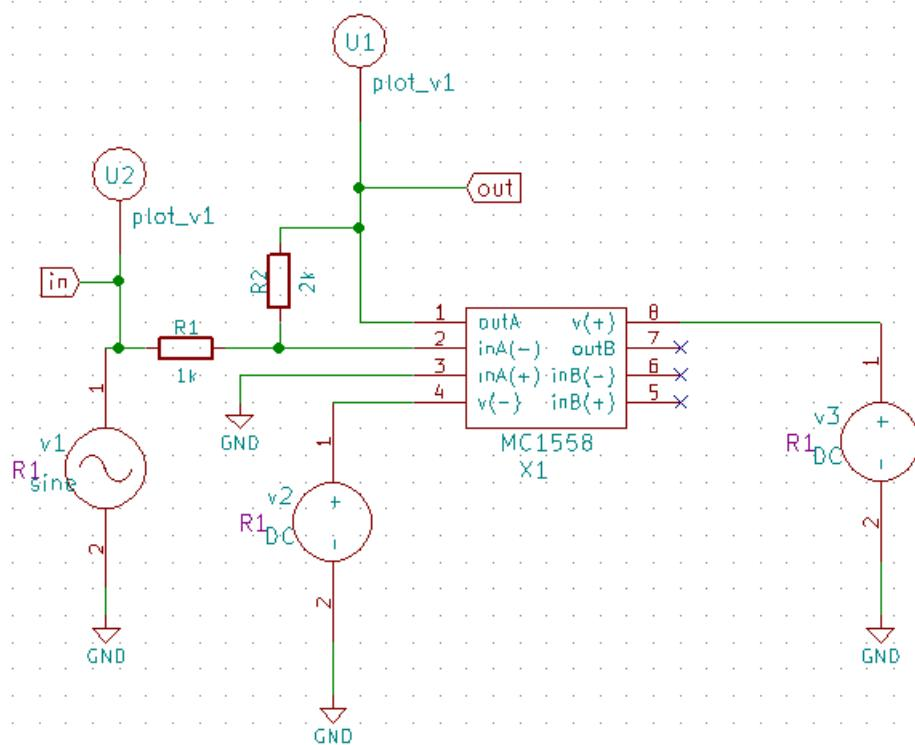
Figure 3.74: MC1558 Test Circuit (Inverting Amplifier)
