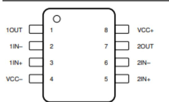
Figure 3.92: TL072 Pin Diagram
