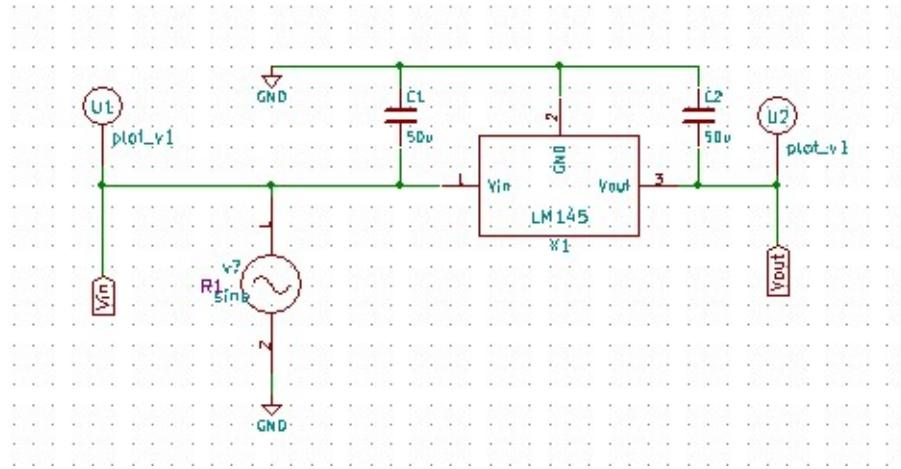
Figure 3.33: LM145 Test Circuit
