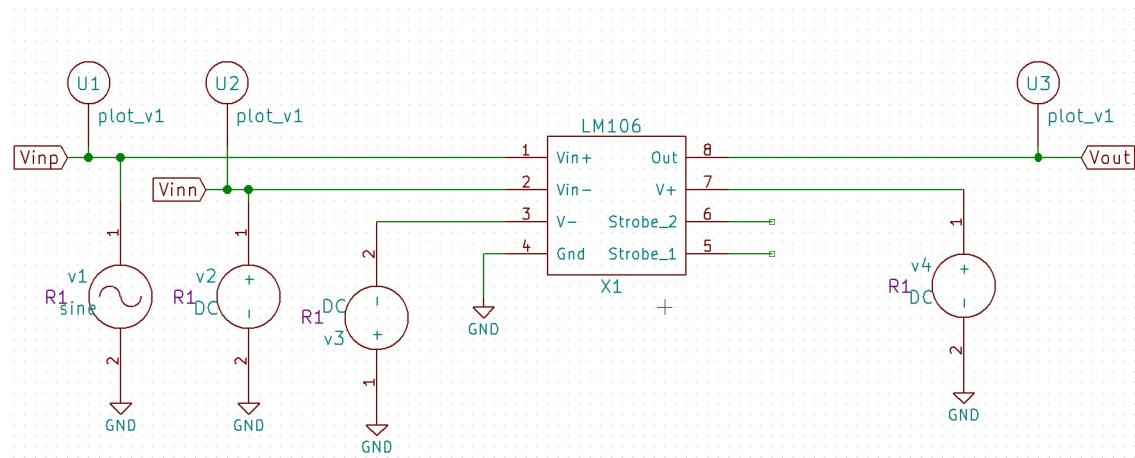
Figure 3.183: LM106 Test Circuit(Voltage Comparator)
