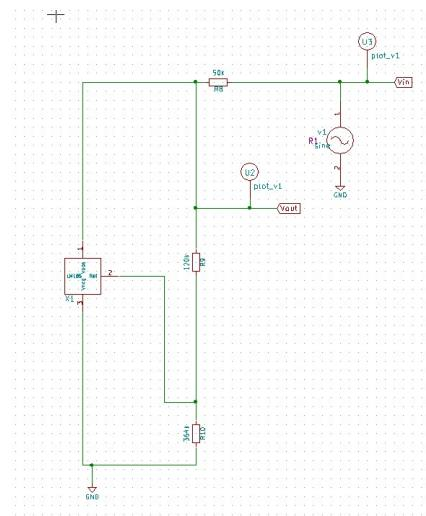
Figure 3.171: LM185 Test Circuit(Voltage Regulator +5V)
