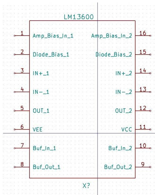
Figure 3.177: LM13600 Pin Diagram
