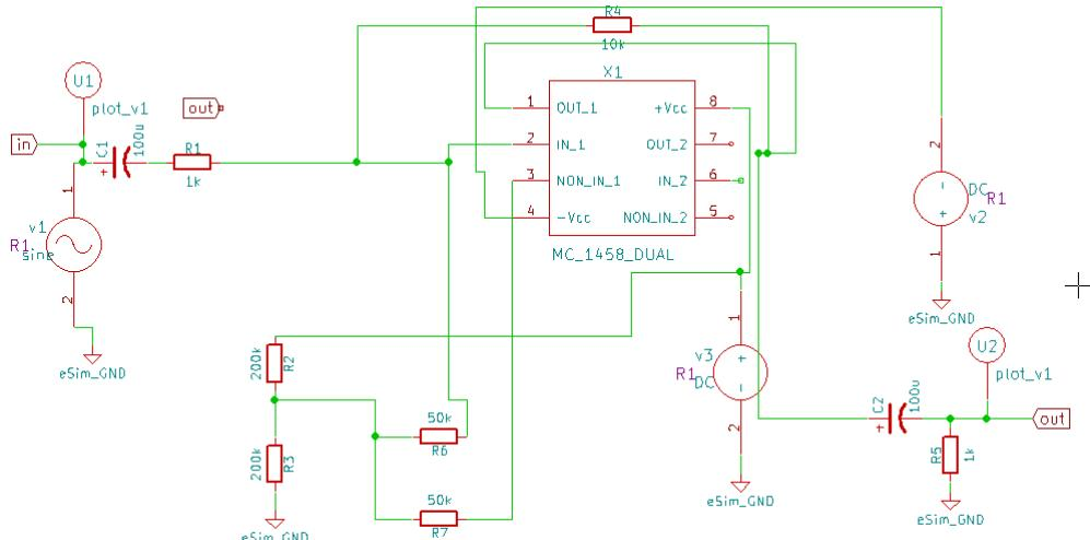
Figure 3.129: MC1458 Test Circuit
