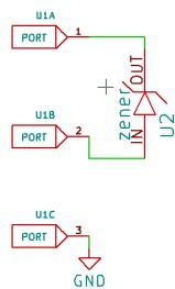
Figure 3.108: LM4040 Schematic of a single pair
