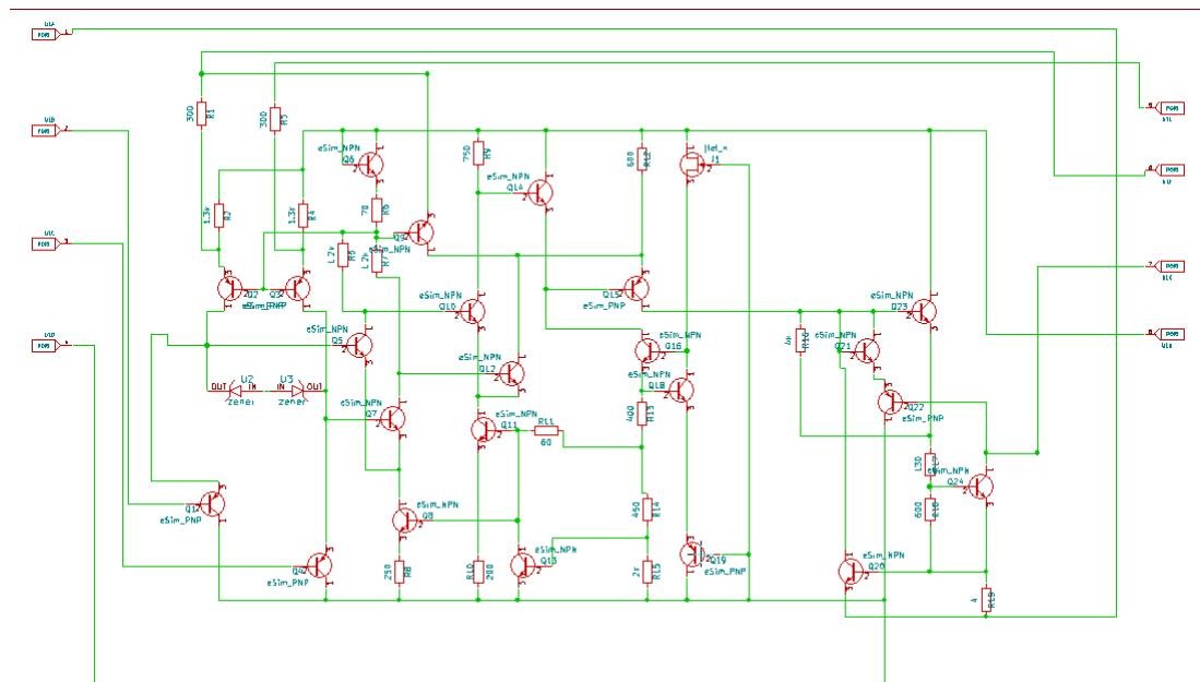
Figure 3.118: LM311 Schematic of a single pair
