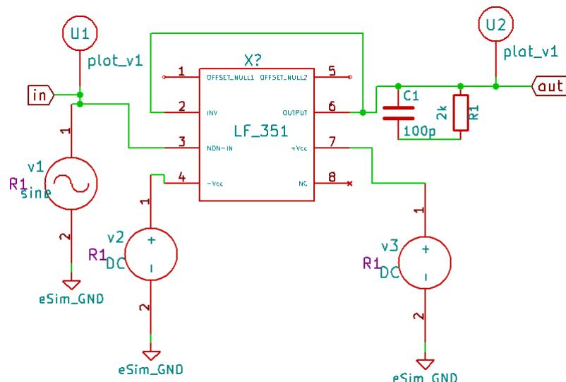
Figure 3.99: LF351 Test Circuit(Voltage Buffer)
