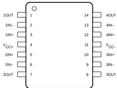
Figure 3.136: LF347 Pin Diagram
