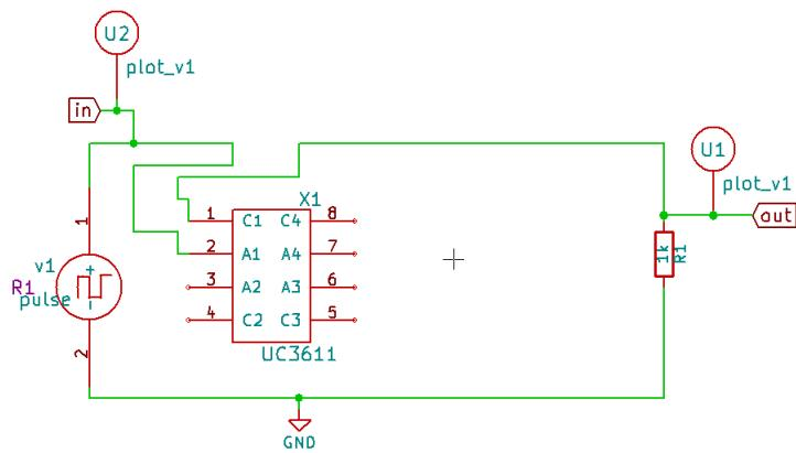
Figure 3.114: UC3611 Test Circuit
