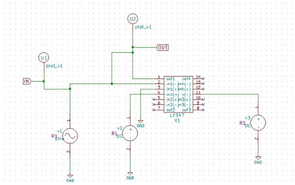
Figure 3.138: LF347 Test Circuit
