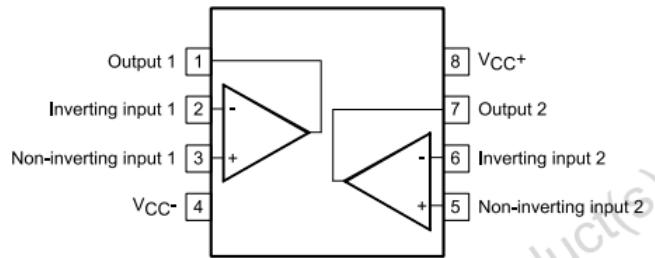
Figure 3.72: MC1558 Pin Diagram
