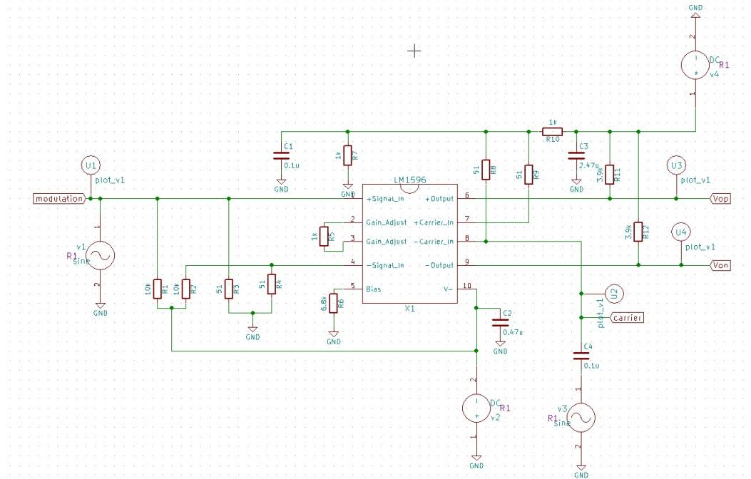
Figure 3.143: LM1596 Test Circuit(Suppressed Carrier Modulator)
