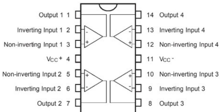
Figure 3.1: TL074 Pin Diagram
