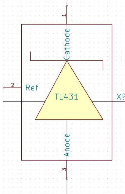
Figure 3.157: TL431 Pin Diagram
