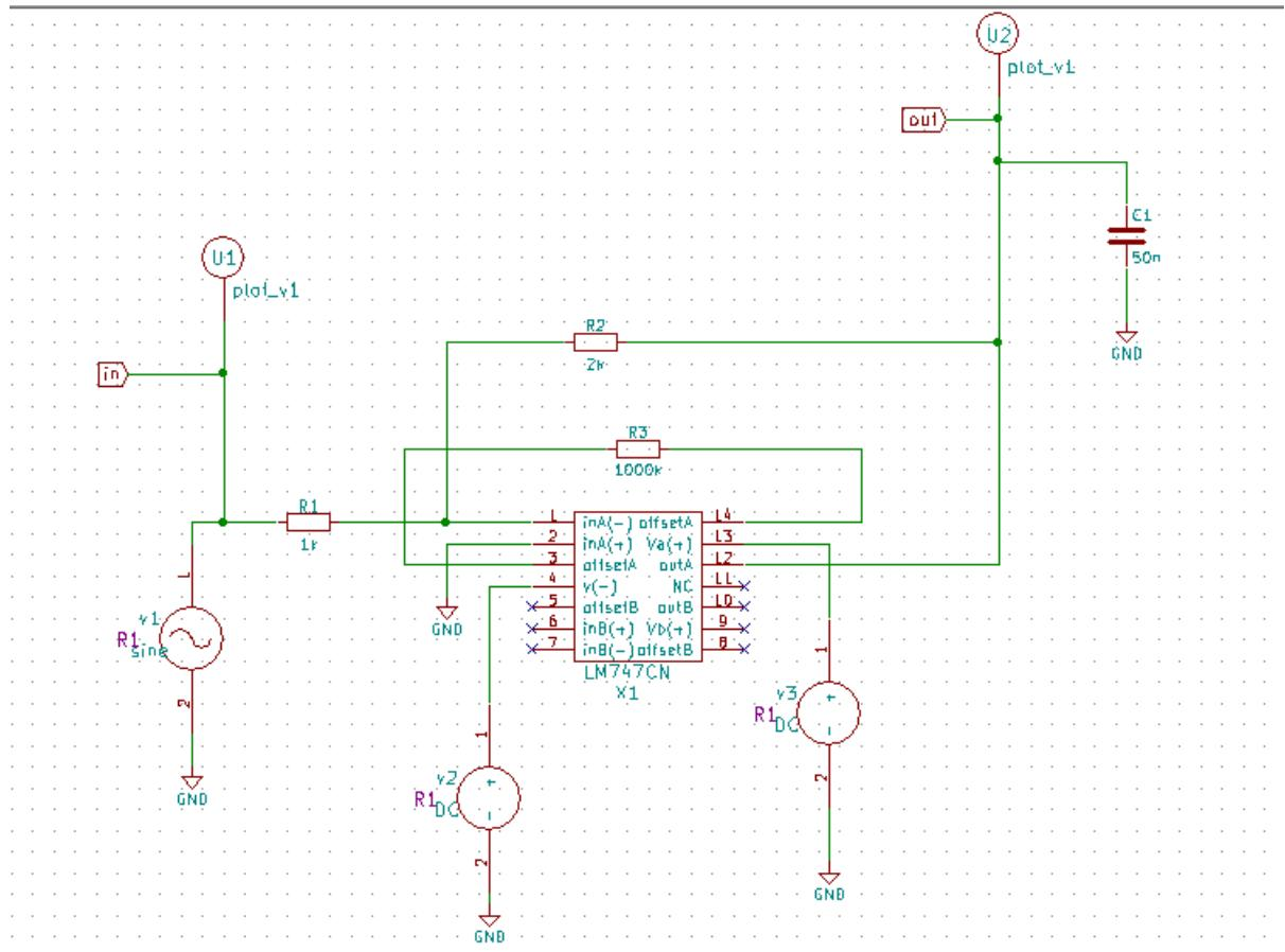
Figure 3.50: LM747 Test Circuit(Inverting Amplifier)
