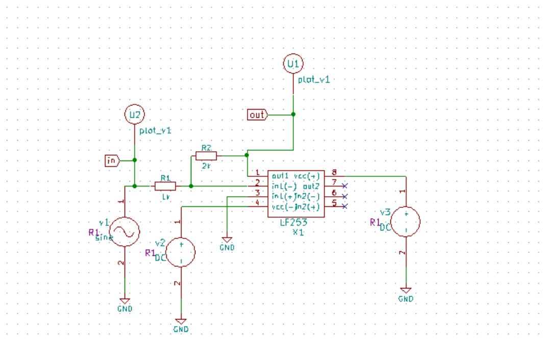
Figure 3.60: LF253 Test Circuit(Inverting Amplifier)
