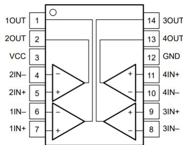
Figure 3.132: LM339 Pin Diagram
