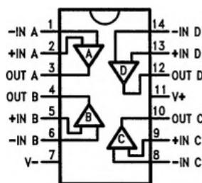
Figure 3.67: LM4136 Pin Diagram
