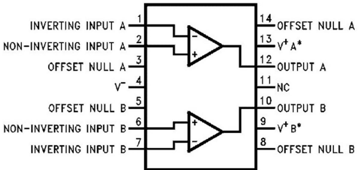
Figure 3.48: LM747 Pin Diagram
