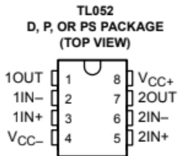
Figure 3.82: TL052 Pin Diagram
