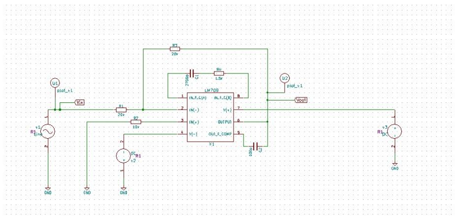
Figure 3.18: LM709 Test Circuit
