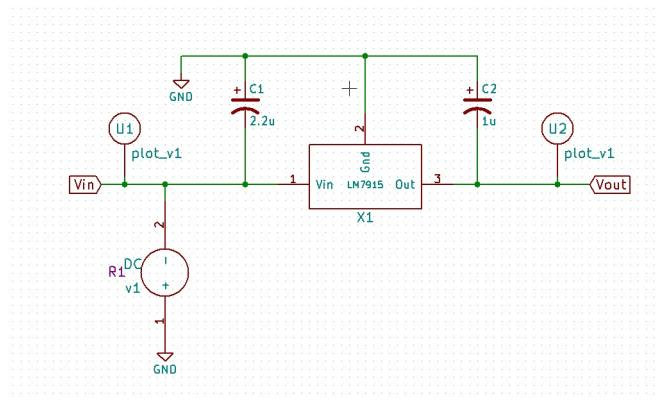
Figure 3.187: LM7915 Test Circuit
