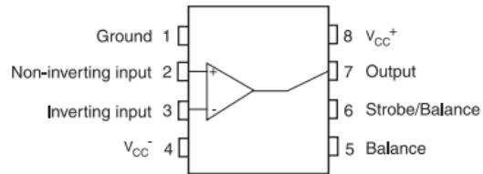
Figure 3.117: LM311 Pin Diagram
