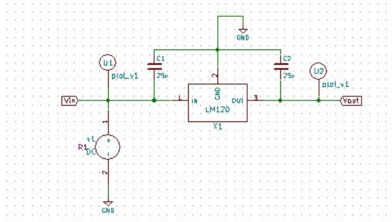
Figure 3.13: LM120 Test Circuit
