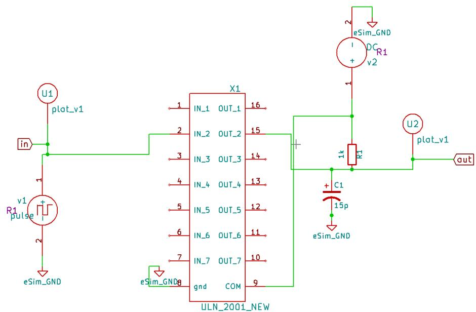
Figure 3.104: ULN2001 Test Circuit(Driver Circuit )
