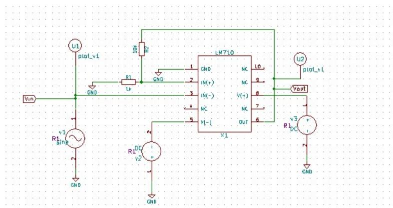
Figure 3.23: LM710 Schmitt Trigger Test Circuit
