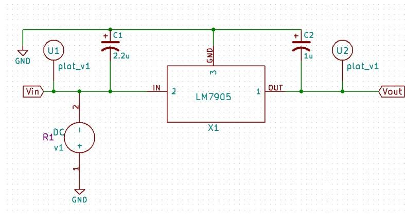
Figure 3.147: LM7905 Test Circuit(Fixed Regulator -5V)
