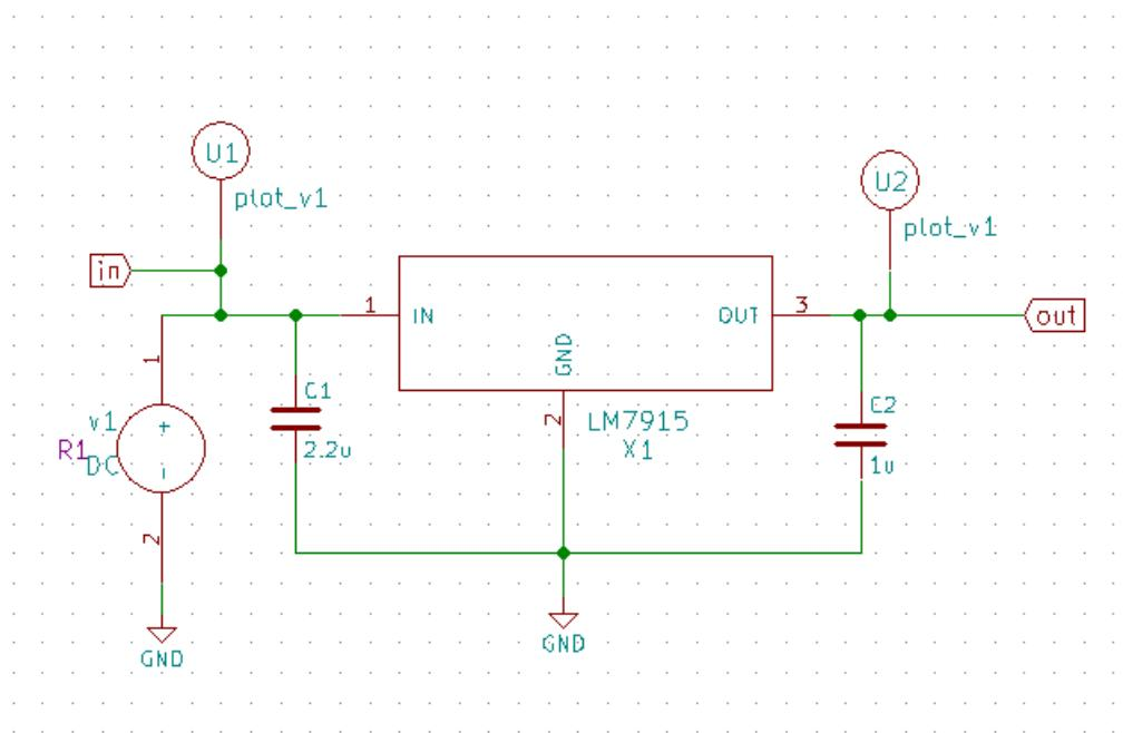
Figure 3.65: L7915 Test Circuit(Voltage Amplifier)
