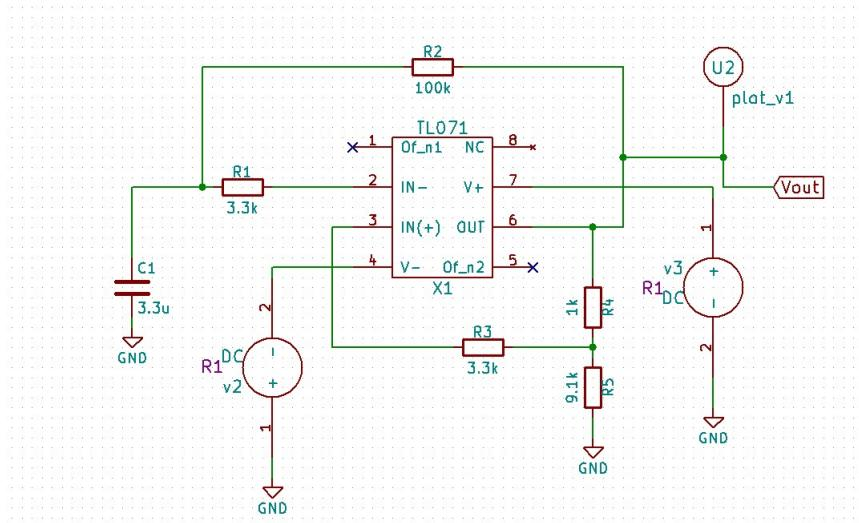
Figure 3.46: TL071 Test Circuit(Square Wave Generator)
