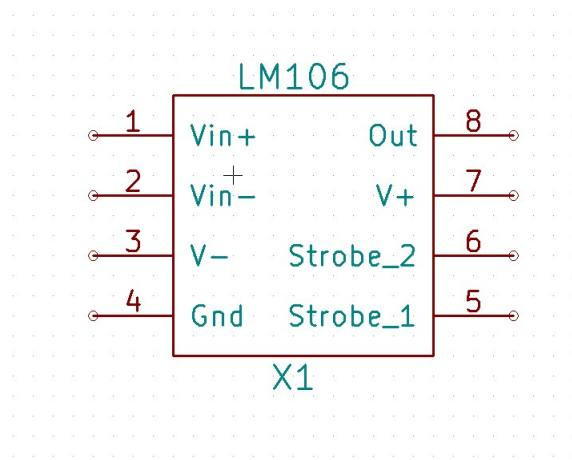
Figure 3.181: LM106 Pin Diagram
