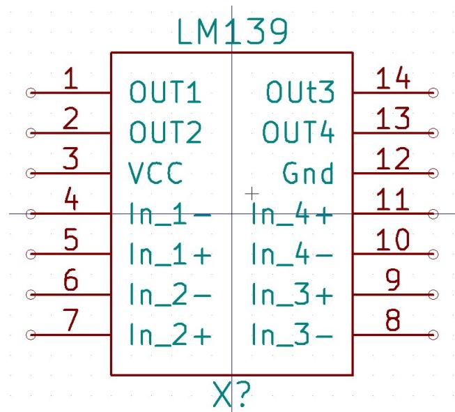
Figure 3.149: LM139 Pin Diagram
