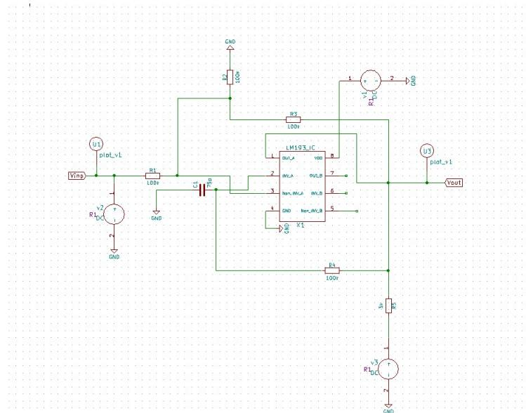
Figure 3.175: LM193 Test Circuit(Square Wave Generator)
