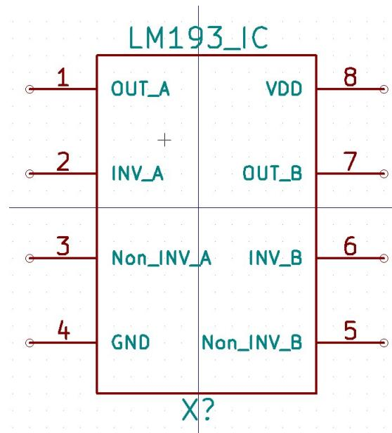
Figure 3.173: LM193 Pin Diagram
