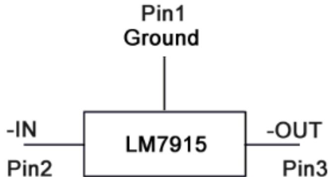
Figure 3.63: L7915 Pin Diagram
