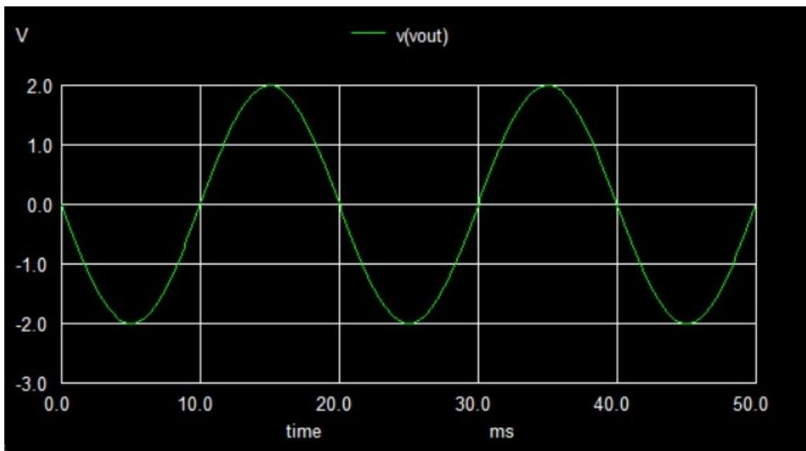
Figure 3.20: Output Unity Gain Inverted Signal
