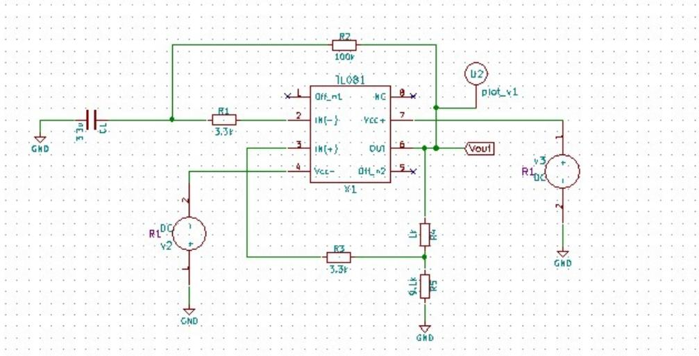
Figure 3.8: TL081 Test Circuit
