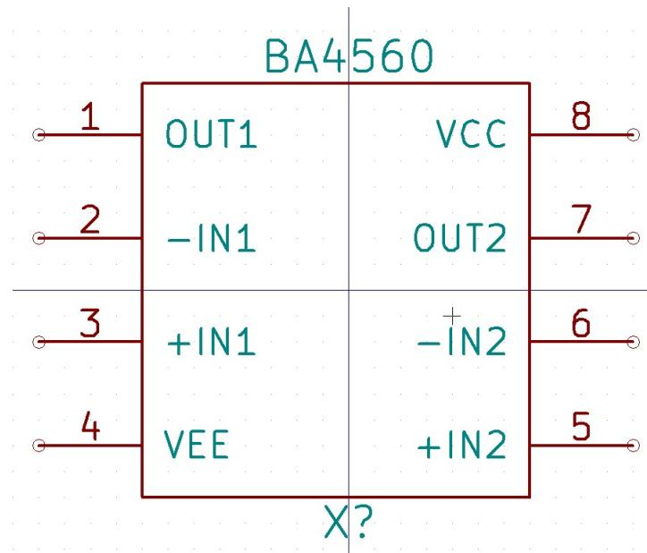
Figure 3.161: BA4560 Pin Diagram
