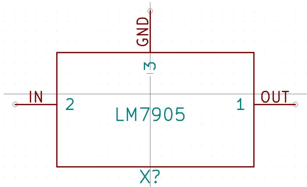
Figure 3.145: LM7905 Pin Diagram
