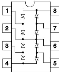
Figure 3.122: UC3610 Pin Diagram
