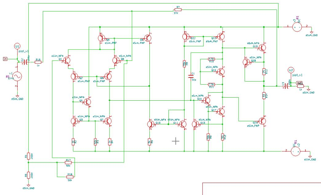
Figure 3.128: MC1458 Schematic of a single pair
