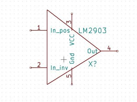
Figure 3.193: LM2903 Pin Diagram
