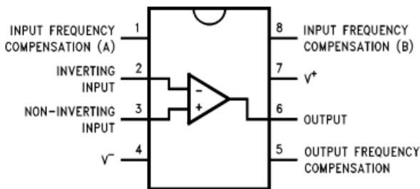
Figure 3.53: Ua709 Pin Diagram
