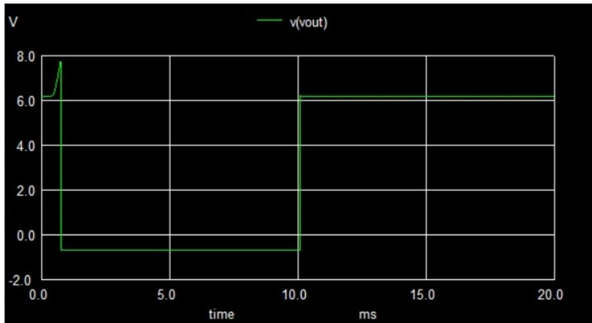
Figure 3.25: Output Signal(Schmitt Trigger)
