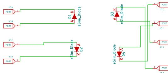
Figure 3.113: UC3611 Schematic of a single pair
