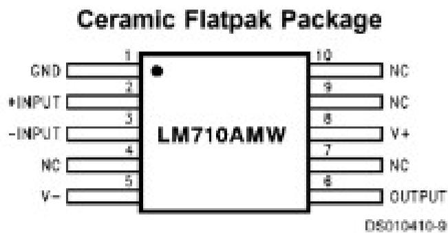
Figure 3.21: LM710 Pin Diagram
