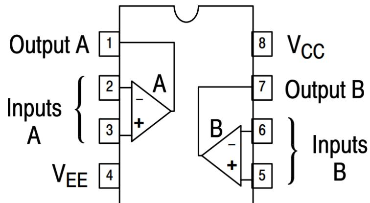
Figure 3.127: MC1458 Pin Diagram
