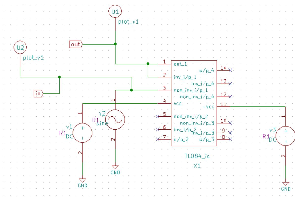
Figure 3.89: TL084 Test Circuit(Voltage follower)
