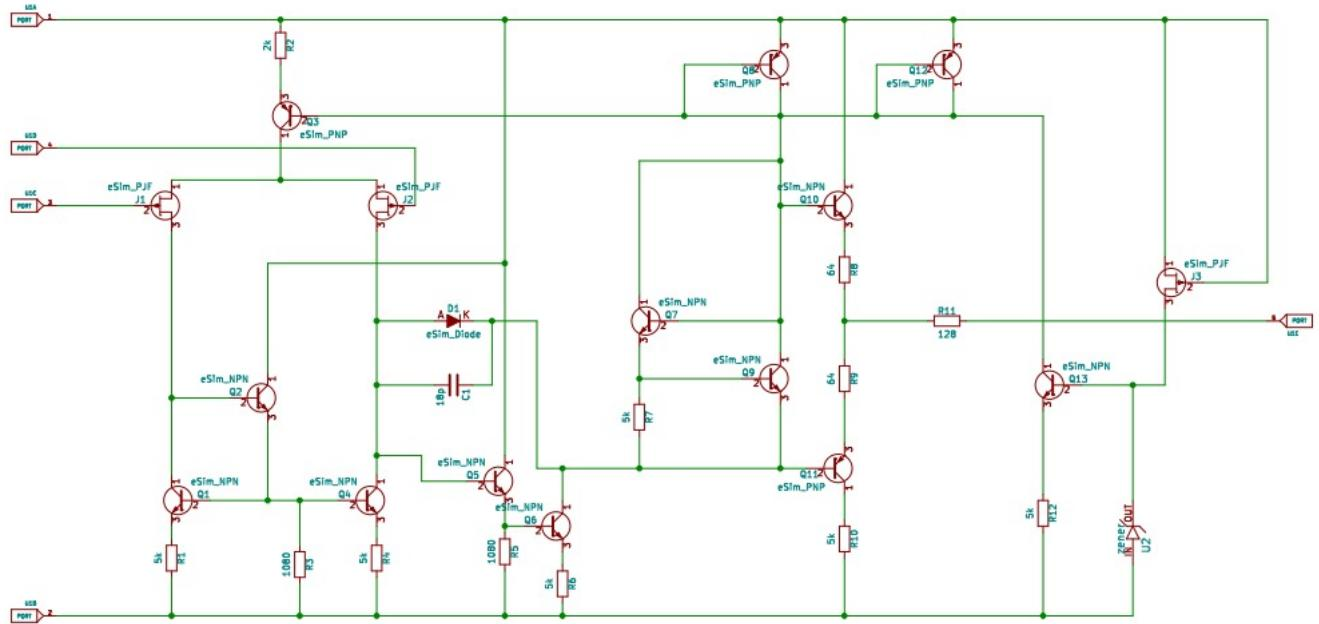
Figure 3.137: LF347 Schematic
