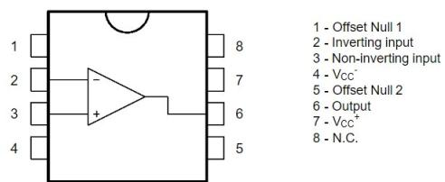
Figure 3.200: TL061 Pin Diagram
