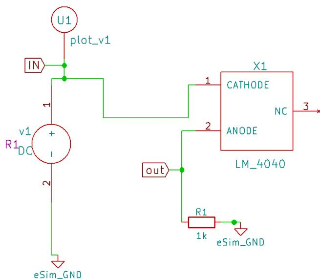
Figure 3.109: LM4040 Test Circuit
