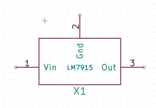
Figure 3.185: LM7915 Pin Diagram
