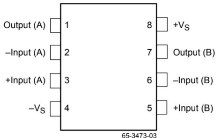
Figure 3.39: RC4558 Pin Diagram
