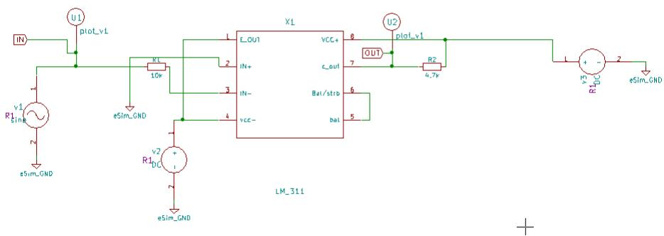
Figure 3.119: LM311 Test Circuit
