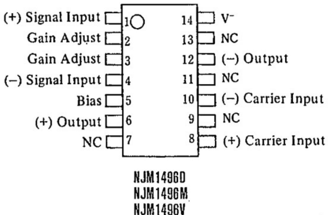
Figure 3.35: NJM1496 Pin Diagram
