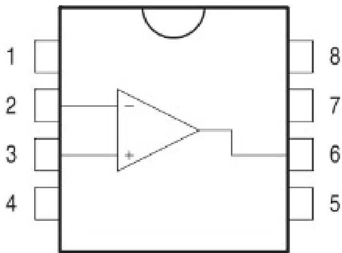
Figure 3.6: TL081 Pin Diagram
