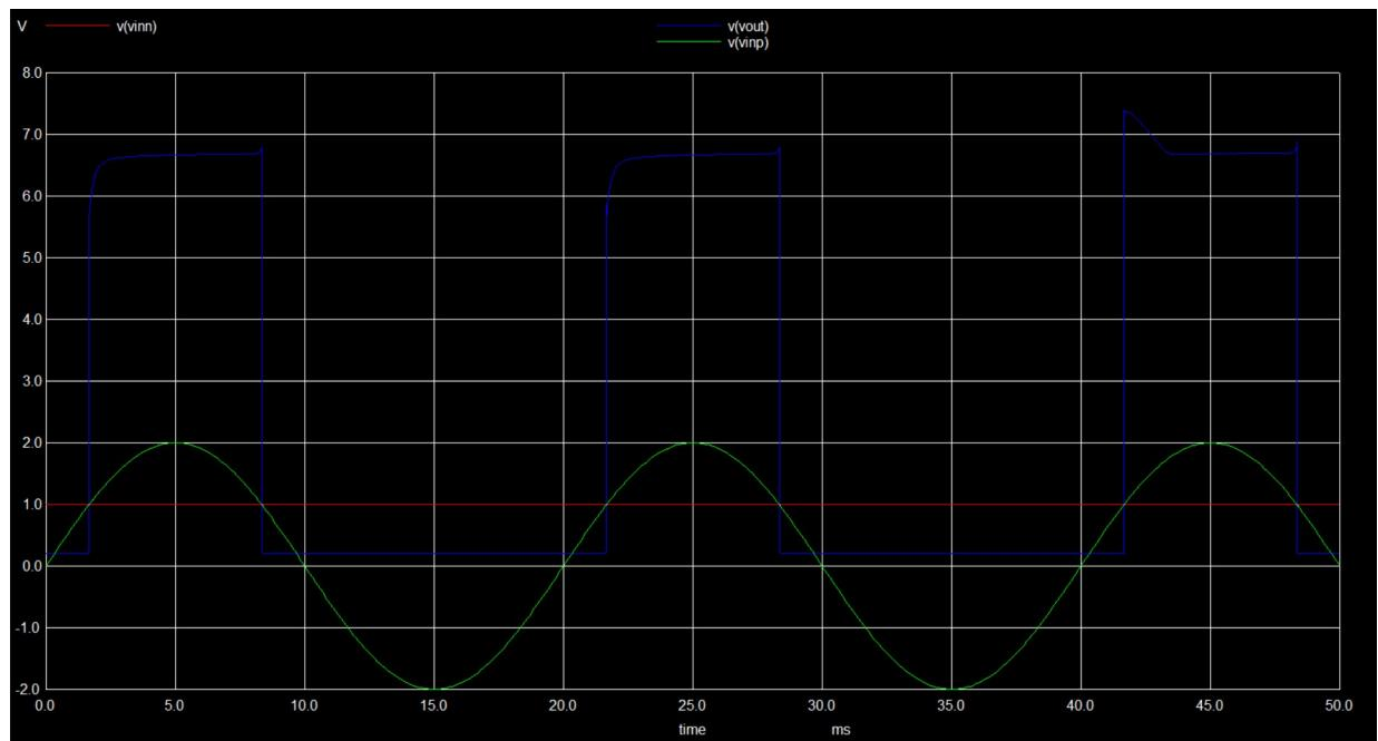
Figure 3.184: Output Voltage Comparator
