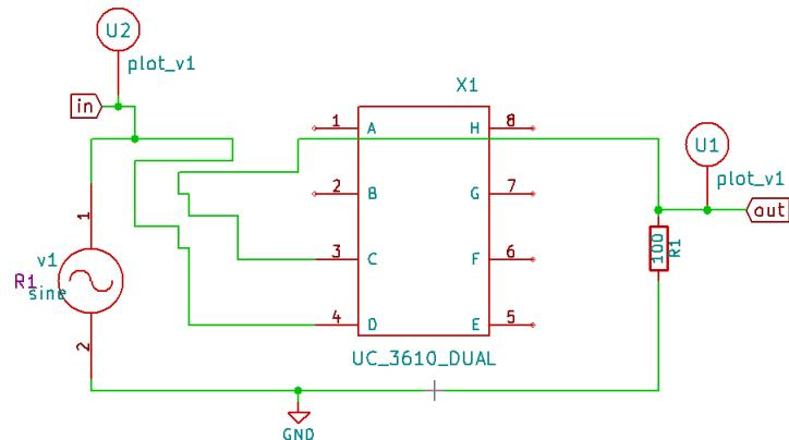
Figure 3.124: UC3610 Test Circuit - Half wave rectifier
