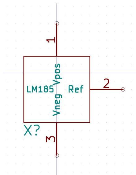
Figure 3.169: LM185 Pin Diagram
