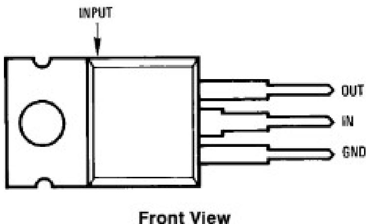
Figure 3.11: LM120 Pin Diagram
