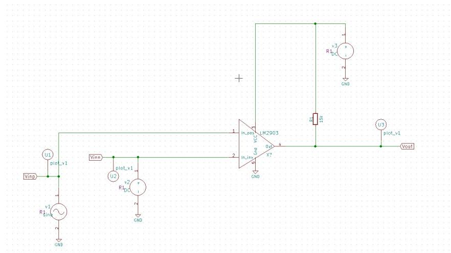
Figure 3.195: LM2903 Test Circuit (Voltage Comparator)
