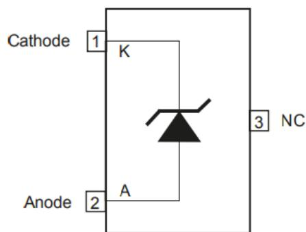
Figure 3.107: LM4040 Pin Diagram
