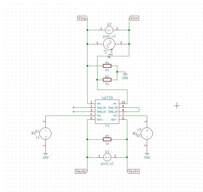
Figure 3.167: UA733 Test Circuit(Non-Inverting Amplifier)
