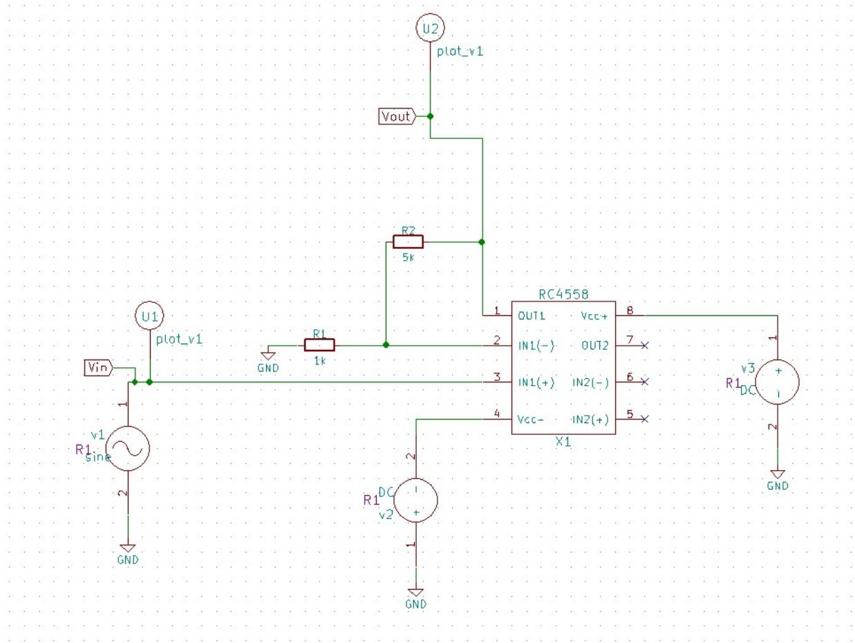
Figure 3.41: RC4558 Test Circuit(Non-Inverting Amplifier)
