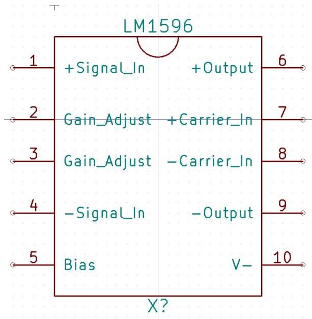
Figure 3.141: LM1596 Pin Diagram
