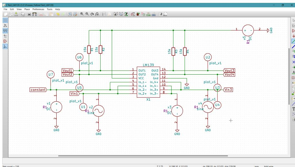
Figure 3.151: LM139 Test Circuit(Comparator)
