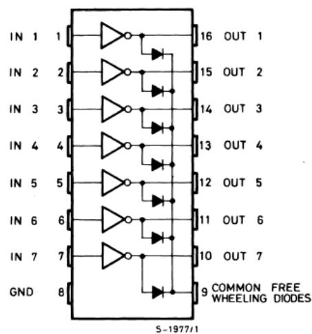
Figure 3.102: ULN Pin Diagram
