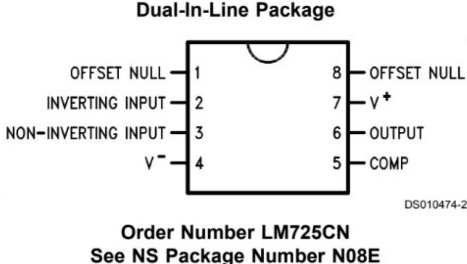
Figure 3.26: LM725 Pin Diagram
