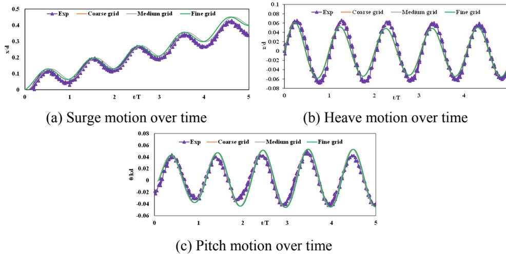
Figure 3: Spatial convergence of freely floating barge with regular waves
