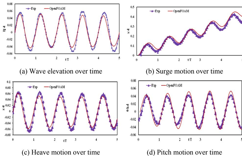
Figure 5: Time histories of motion trajectories of freely floating barge with regular waves
