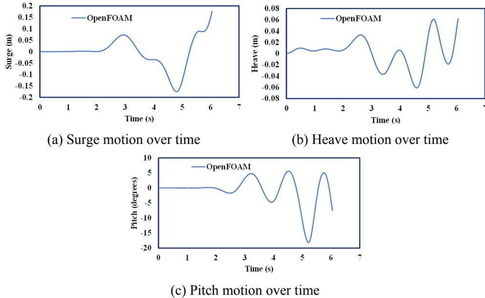
Figure 8: Time histories of motion trajectories of freely floating barge with irregular waves
