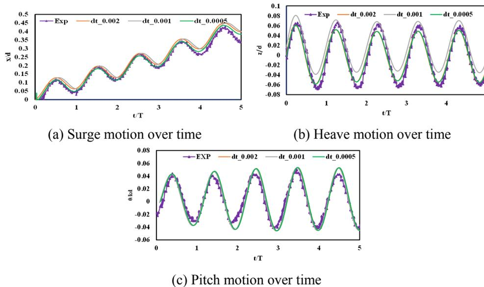
Figure 4: Temporal convergence of freely floating barge with regular waves
