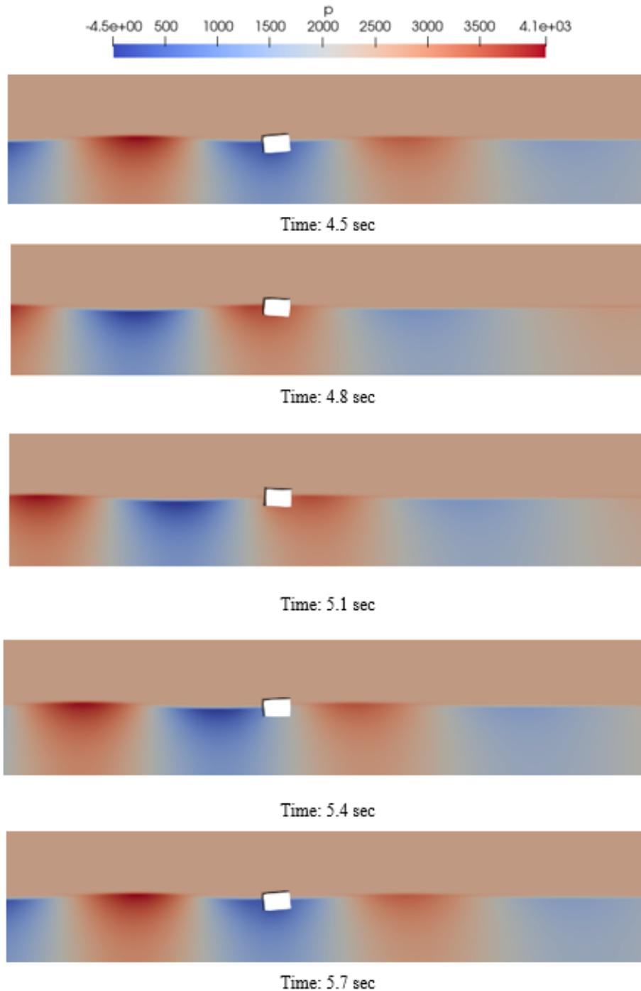
Figure 6: Different time instants of the interaction of regular waves with freely floating barge (pressure)
