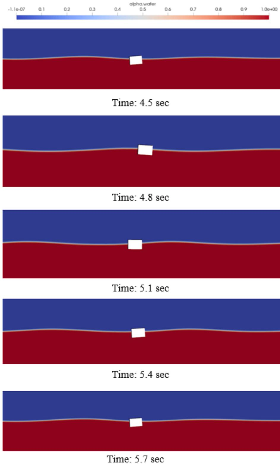
Figure 7: Different time instants of the interaction of regular waves with freely floating barge (alpha water)
