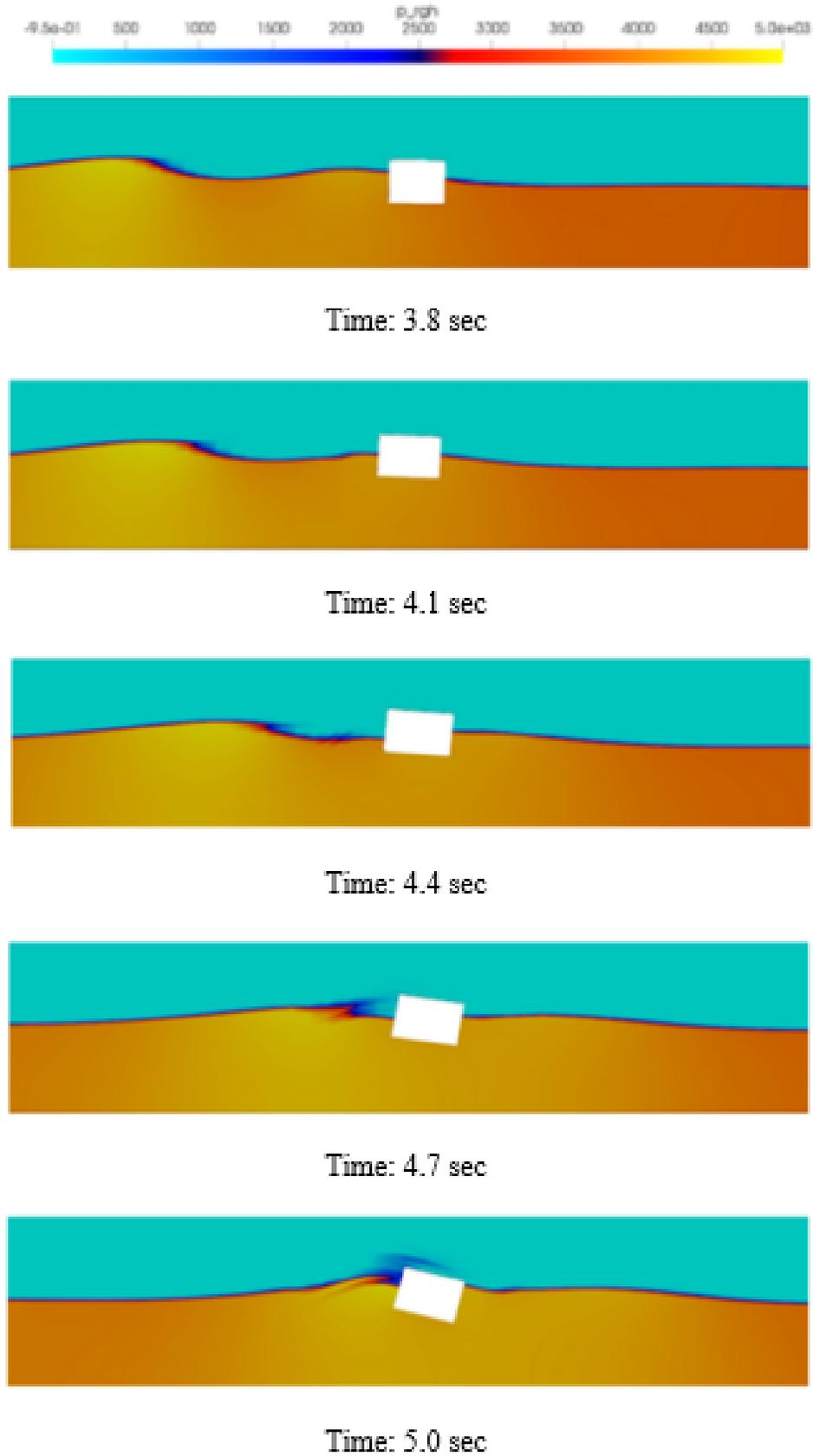
Figure 10: Different time instants of the interaction of irregular waves with a freely floating barge (pressure)
