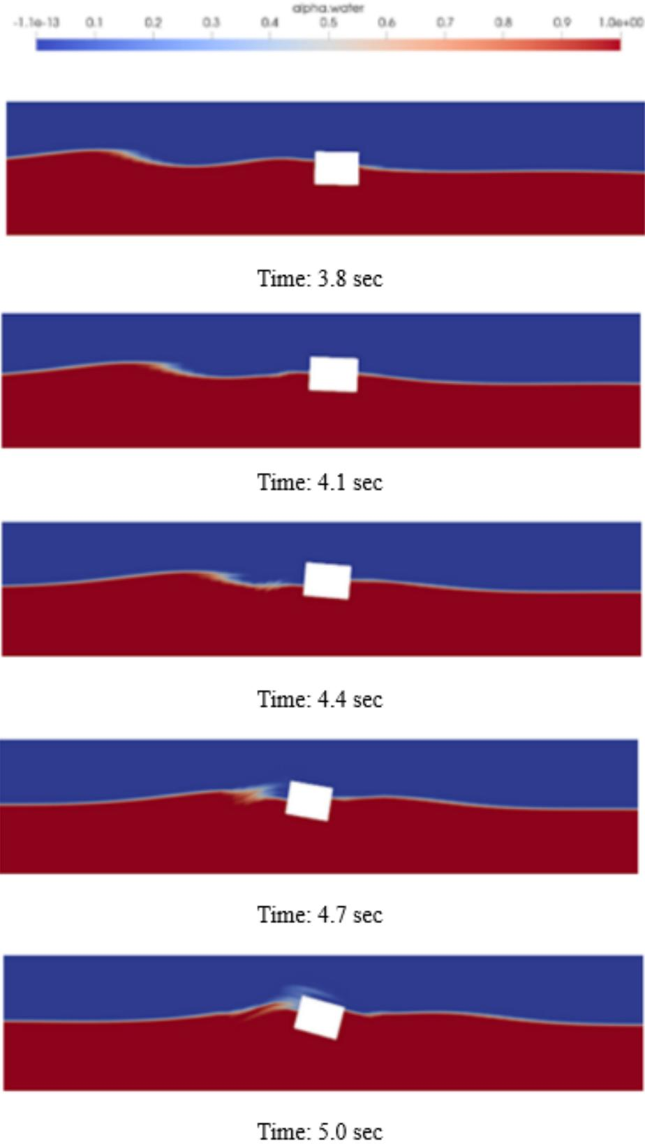
Figure 9: Different time instants of the interaction of irregular waves with freely floating barge (alpha water)
