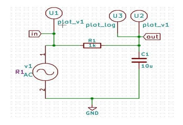
Fig 1. Low pass filter circuit
