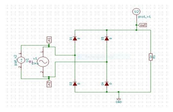
Figure 1: Fullwave Bridge rectifier
