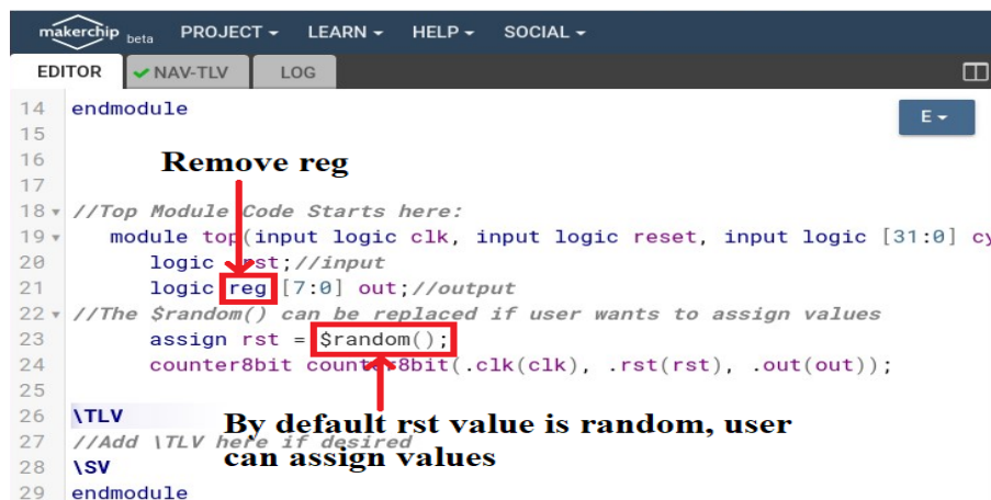
Figure 11.18: Top level verilog code
