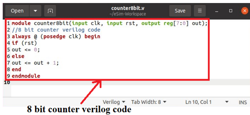
Figure 11.9: 8 bit Counter verilog code
